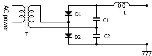
Figure 1. Schematic of the full wave voltage doubler
