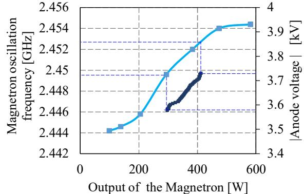
**Figure 5.** Characteristics of the magnetron (upper trace: oscillation frequency vs. output power, lower trace: anode voltage vs. output power based on the full wave voltage doubler)
