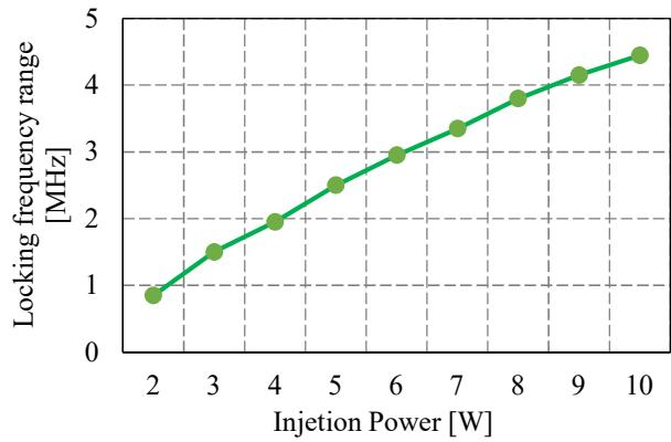
**Figure 4.** Injection power vs. lock frequency range
