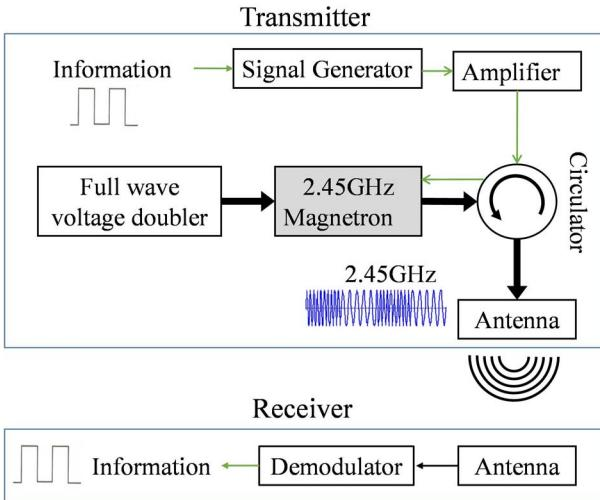
**Figure 2.** FSK system block diagram
