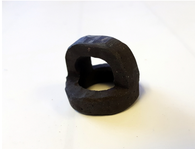
Figure 12a: A cast core for an experimental current-controlled inductor.
