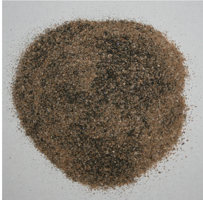
Figure 6a: Magnetite sand as initially harvested.
