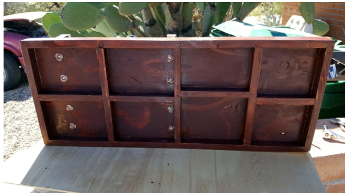
Figure 16a: The base of my ball mill is a framed plywood deck, reinforced with ribs. The underside of the base is visible here.
