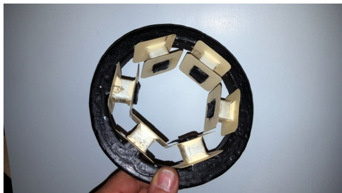
Figure 18g: A complete set of cardboard coil bobbins are temporarily installed on the stator to test for proper fit.
