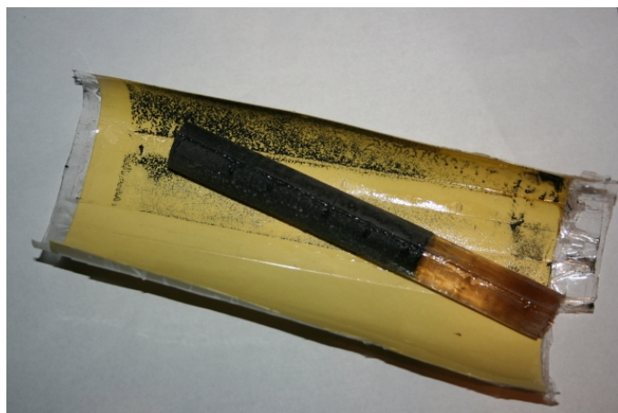
Figure 8b: A bar of cast magnetite sand emerges from the a paper mold. Note the packing-tape-plastic lining in the mold.
