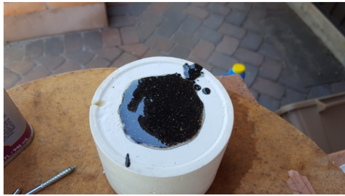
Figure 13d: Black sand and resin slurry is spooned into the mold.
