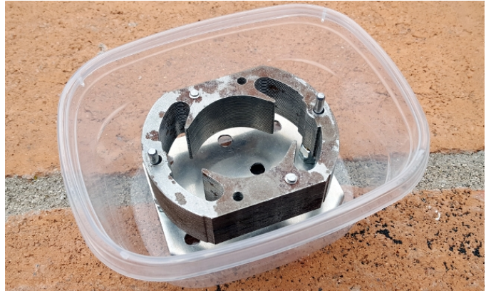
Figure 17e: The field frame and registration fixture in the mold container, awaiting the silicone rubber.
