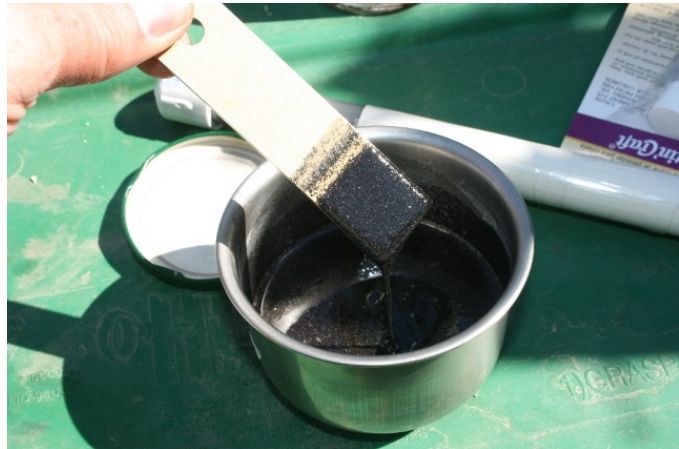
Figure 8a: Magnetic structures can be cast with a slurry comprised of refined magnetite sand and a polyester resin binder.
