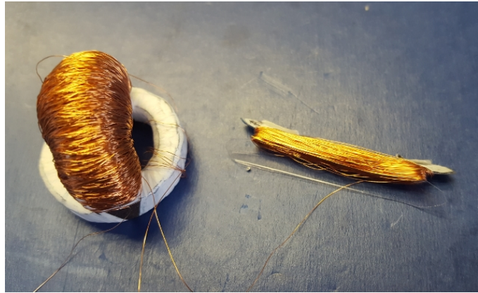
Figure 12b: Here, the control winding (left) is being added to the cast core. Supply wire is stored on a long, narrow, plastic shuttle (right). The shuttle is sufficiently narrow to allow it to pass through the bore of the casting.
