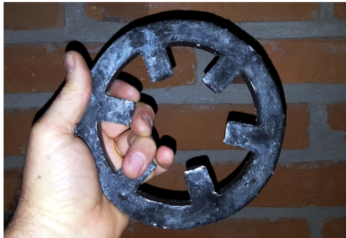
Figure 18c: The finished stator, as extracted from the mold.
