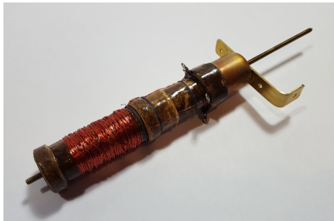
Figure 11f: Loop-sticks can easily be fashioned in any size. The cap at the head of this loop-stick is a 3/4-inch copper fitting.
