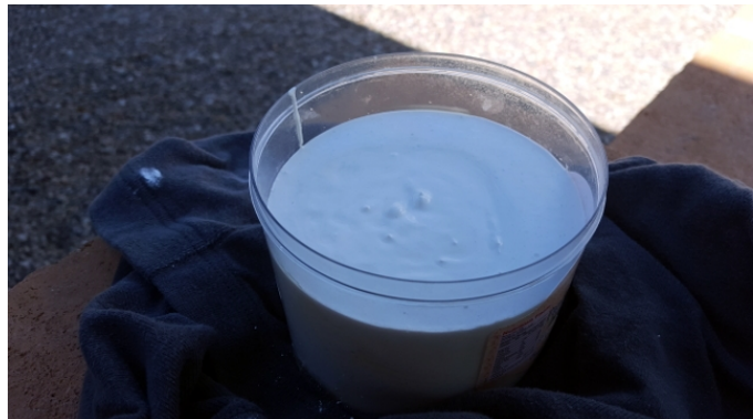
Figure 13b: Plaster of Paris is poured onto the “positive.”
