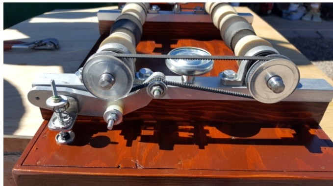
Figure 16c: Detail of the pulleys and belt that link the roller shafts. Beneath the left pulley lies a tensioning mechanism. A compression spring applies downward force to the left side of a pivoting arm. On the right side, the arm is fitted with an idler wheel which applies pressure to the exterior of the belt. Tension in the belt is adjustable by manipulating the nut above compression spring.
