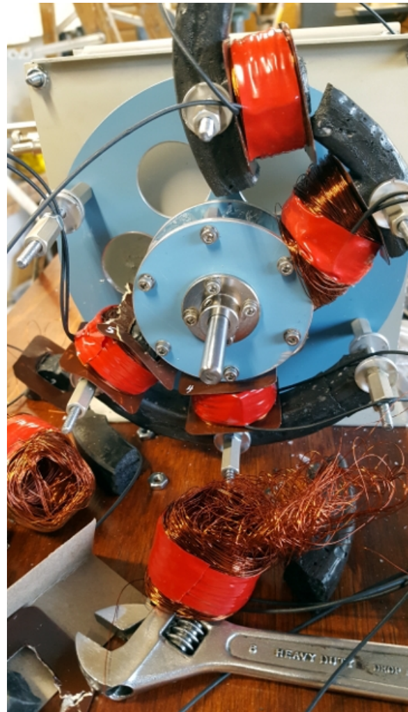
Figure 18o: The first alternator exploded and essentially gutted itself.
