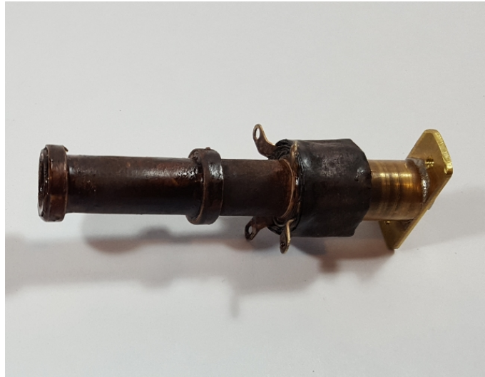
Figure 11c: A close-up of the loop-stick body. Note the wound paper flanges (to confine the coil windings), the wound paper terminal block, and the brass cap, which engages the threads on the stem of the slug.
