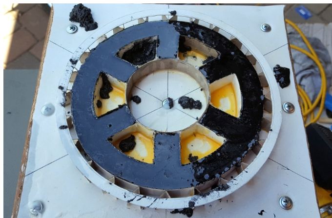
Figure 18b: The stator mold, filled with processed-brake-turnings-and-resin mix.
