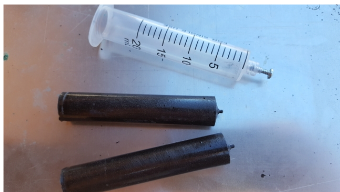
Figure 8d: Test bars, used for evaluation of grain packing methods, cast in a syringe body.
