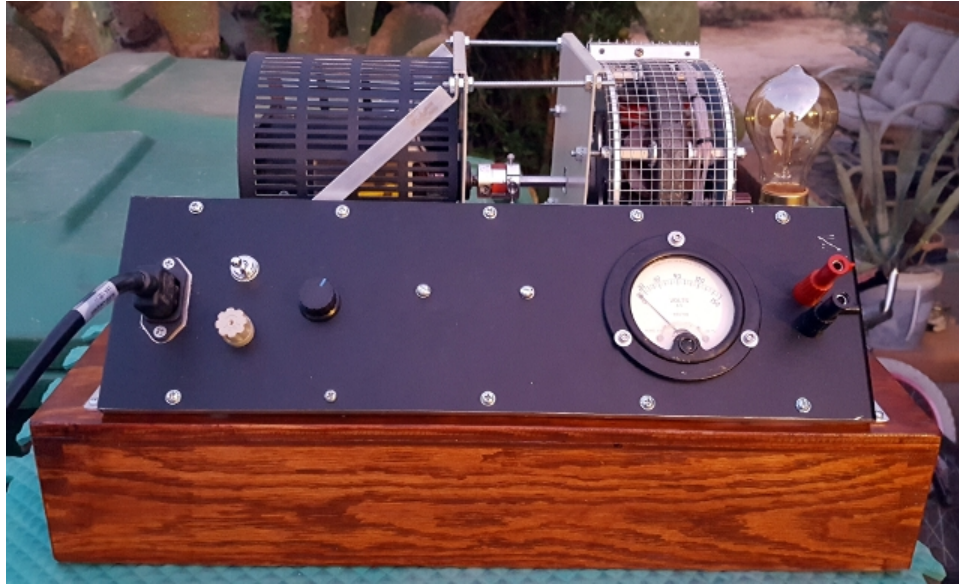
Figure 18v: The final version of the alternator test stand. At the rear (left) is the drive motor. At rear (right) is the improved alternator adjacent a 60-watt incandescent load. In the front is a control panel with a power switch, motor speed control, an AC voltmeter, and binding posts to which external loads or instrumentation can be connected.
