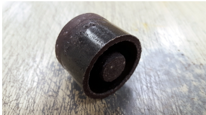
Figure 13e: A beautiful magnetite pot core emerged from the mold.
