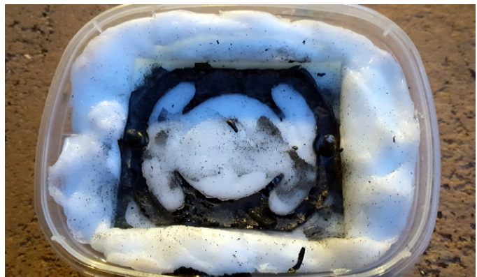
Figure 17g: A newly cast field frame, hardened in the silicone mold.
