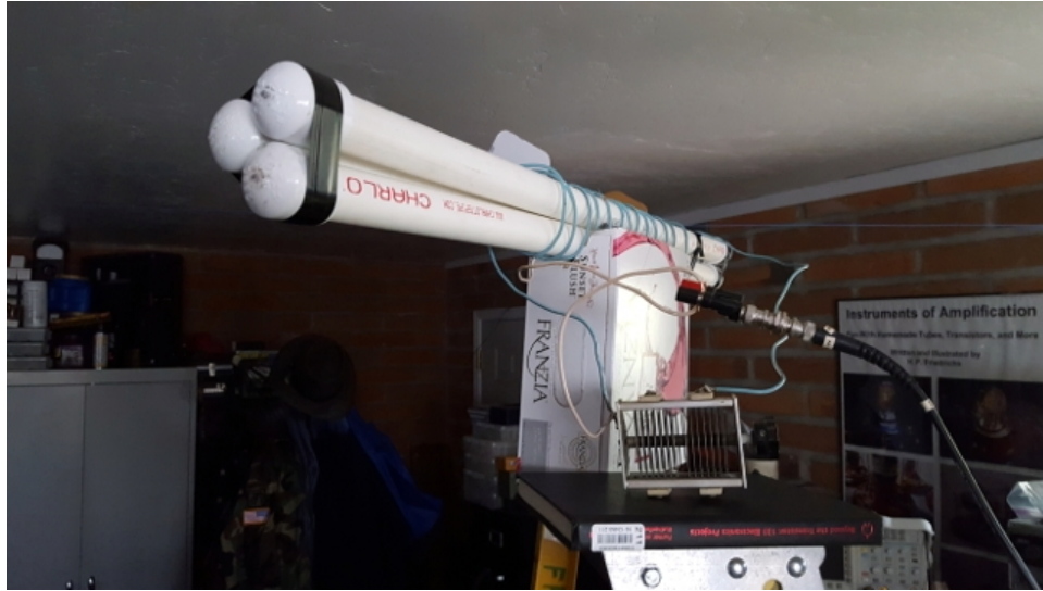
Figure 15b: The core of this transmitting antenna contains three PVC tubes and three times the volume of magnetite as the antenna in Figure 15a.
