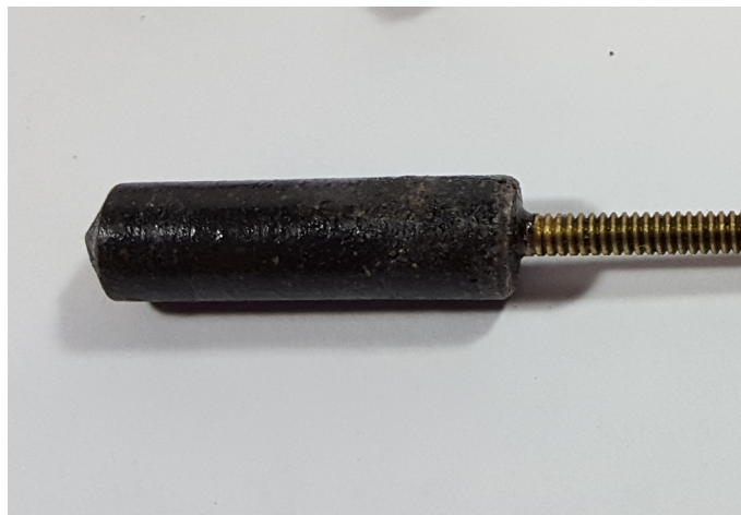
Figure 11b: Close-up of the cast black-sand slug and threaded brass stem.
