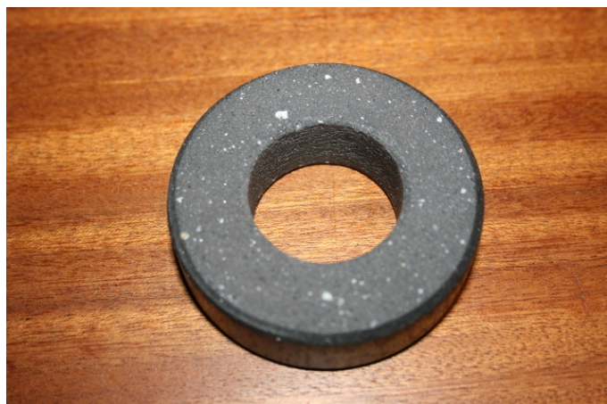
Figure 10b: Close-up of a black sand toroid.
