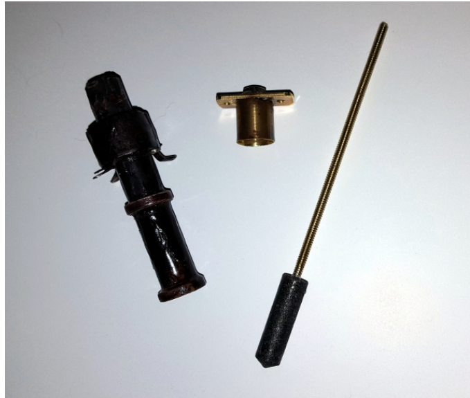
Figure 11a: Parts of an adjustable loop-stick include the body (on which a coil is ultimately wound), a cap, and an adjustable slug. These parts were fabricated as described in the text.
