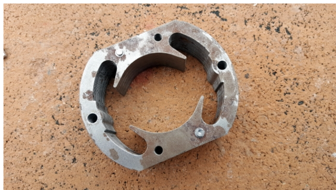
Figure 17b: This structure, comprised of stamped steel laminations, stacked and riveted together, comprised the physical frame and core for the field coils in the original motor.
