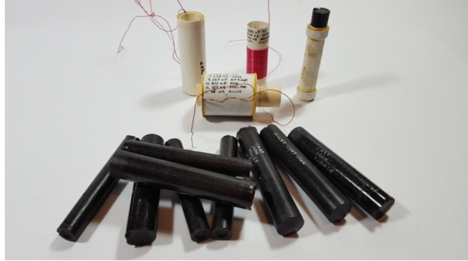
Figure 8.0e: Multiple examples of test bars and test coils.
