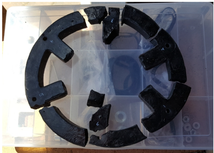
Figure 18q: Failure of the alternator resulted in complete destruction of the stator. Remarkably, this level of damage was still repairable.
