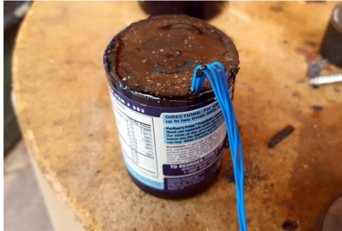
Figure 14c: A vitamin pill bottle is a practical mold in which to cast this transformer.
