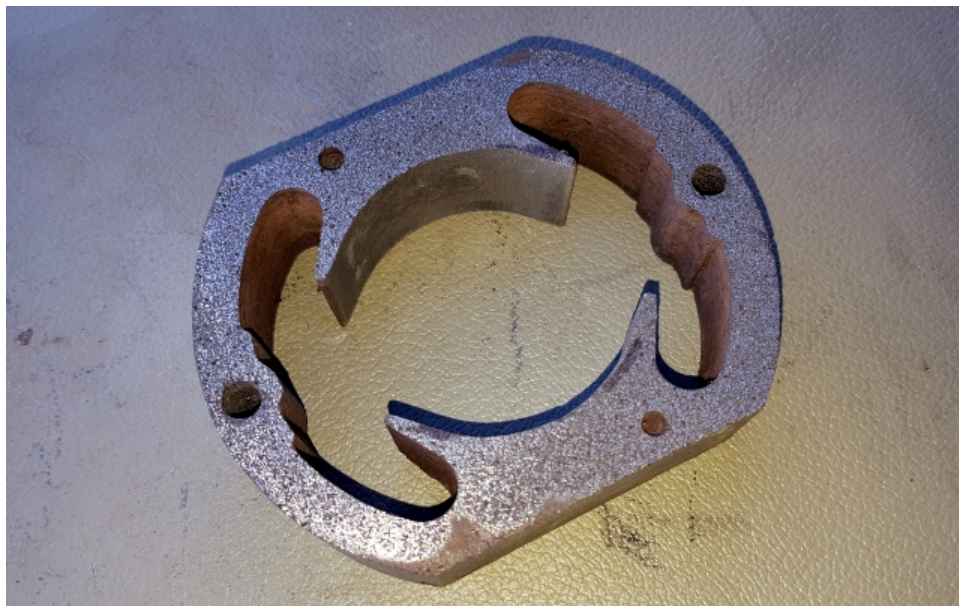
Figure 17i: The new field frame, cleaned and polished.
