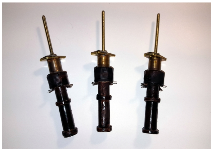
Figure 11d: The fabrication process described in the text is repeatable. Here, three loop-stick “sisters” await the winding of their coils.
