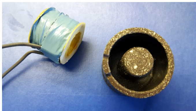
Figure 13f: The coil assembly, ready for installation in the core. Note the notches in the rim of the core to allow egress of the coil's leads.
