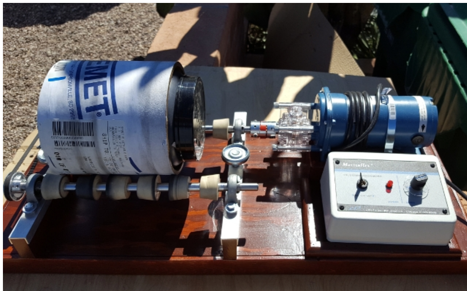
Figure 16g: The completed ball mill in operation.
