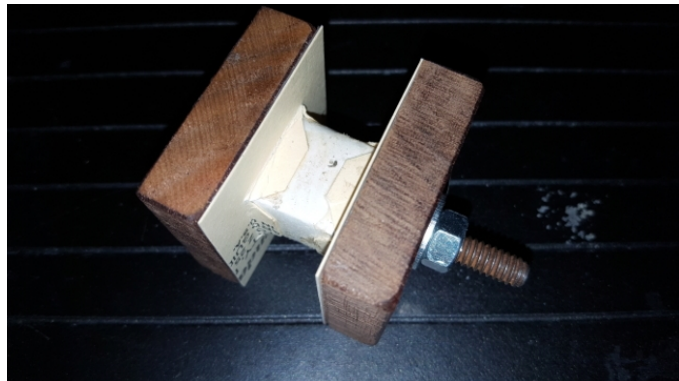
Figure 18f: A cardboard coil bobbin nearing completion.
