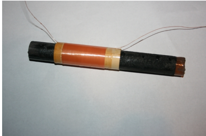
Figure 8c: Cast bar, trimmed, fitted with paper sleeve and coil.
