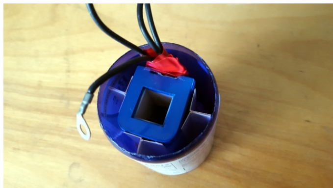
Figure 14f: The coil assembly has been inserted into a vitamin pill bottle and awaits the casting process.
