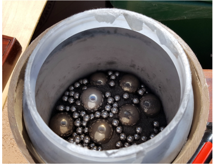
Figure 16f: The interior of the ball mill's drum. Loose ball bearings of assorted sizes grind and pulverize brake drum turnings into usable form.
