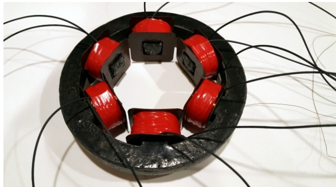
Figure 18j: Finished rotor coils installed on the stator.
