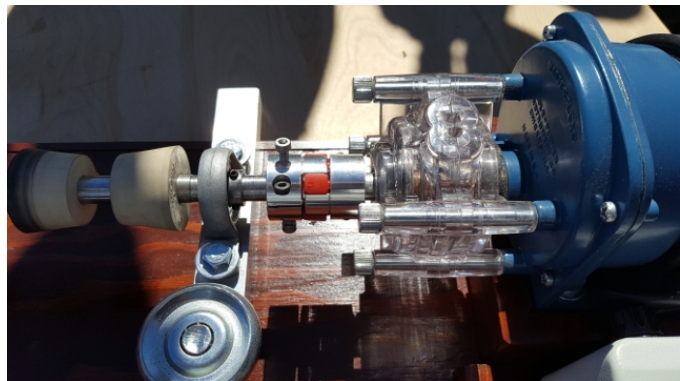
Figure 16e: At the rear of the mill, a jaw-style coupler joints the shaft of the the gear motor and the rear roller shaft. Also visible is one of the metal garage door rollers (bottom) that is used to prevent the revolving drum from wandering off the rubber drive rollers.
