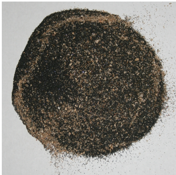
Figure 6b: Magnetite sand, partially refined.
