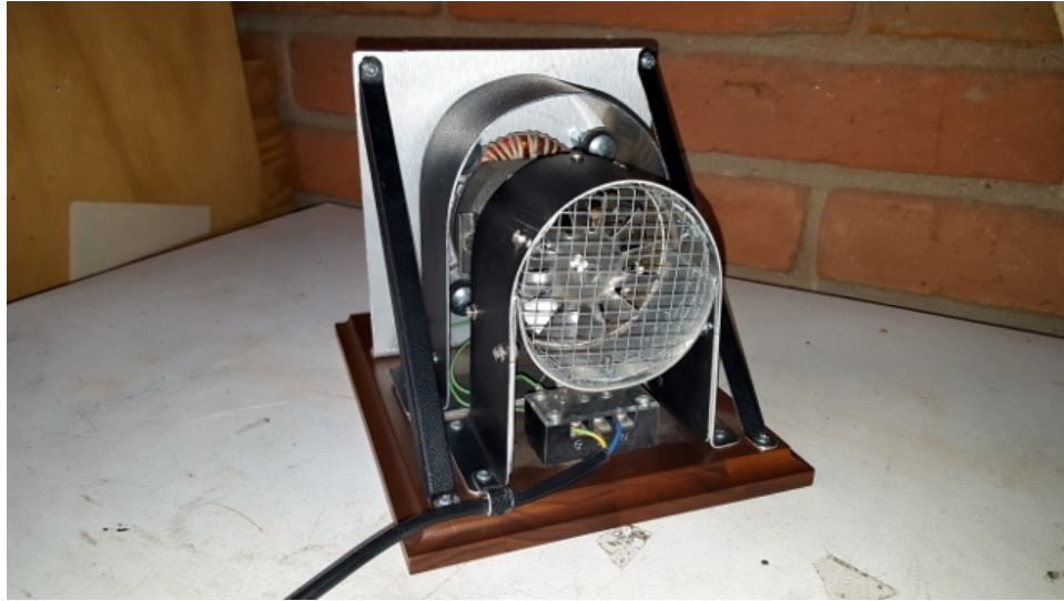
Figure 17l: For demonstration purposes the motor was mounted to a “test stand,” complete with finger guards, shields, and properly grounded wiring.
