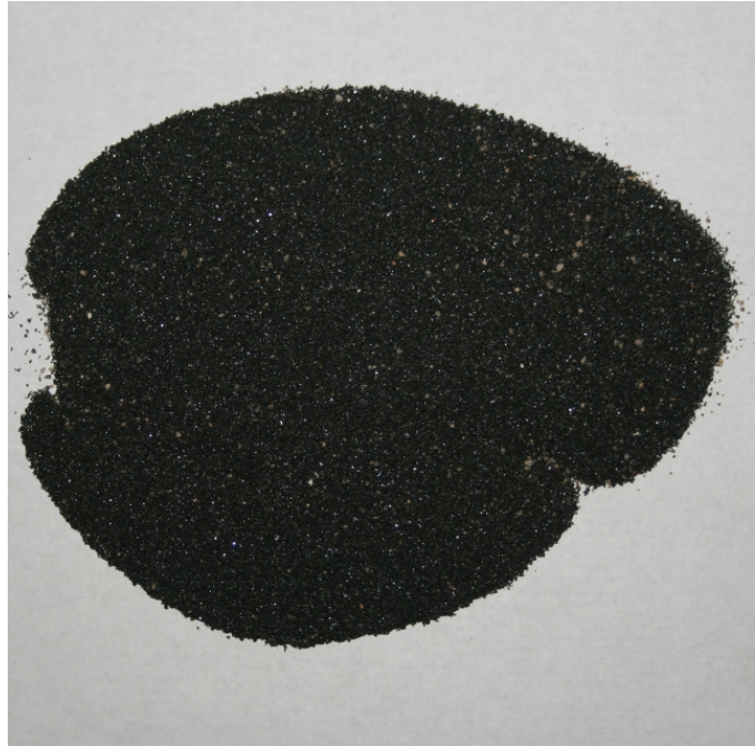
Figure 6c: Magnetite sand after several refinement cycles.
