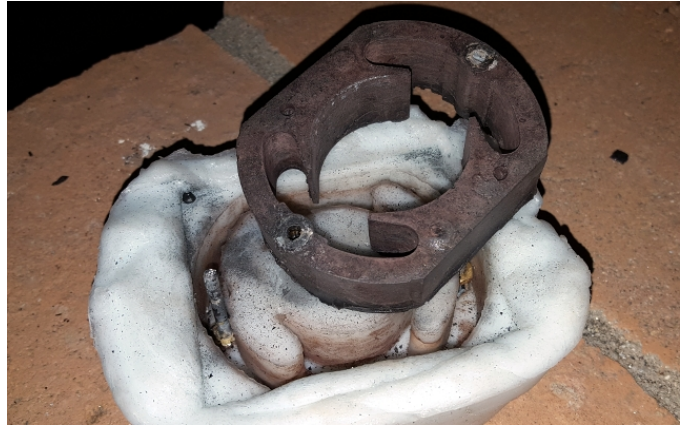
Figure 17h: A newly cast field frame, emerging from the mold.
