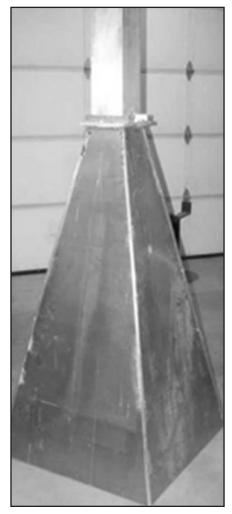
Figure 5. CP horn antenna using all-aluminum construction.
