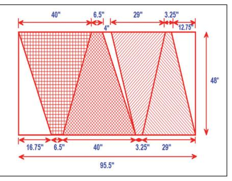
Figure 2. Pattern for linear horn construction from a single sheet  $(48" \times 96")$  of material.
