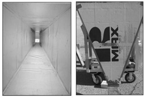
*Figures 3 & 4. Inside of foam/aluminum horn with taped seams. Outside of low-cost horn antenna.*
