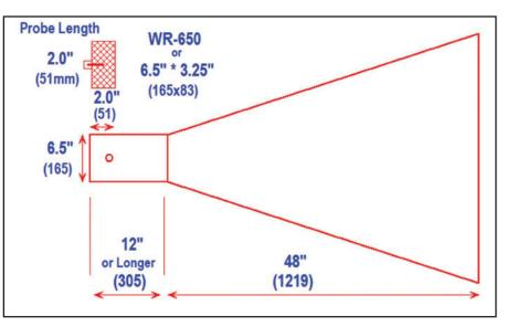
Figure 1. 23-cm linearly polarized 20-dBi horn antenna.
