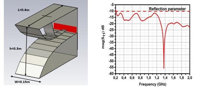
Fig. 4. K Antenna and reflection coefficient magnitude
