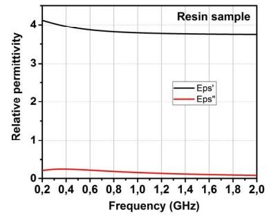
Fig. 7. Real part ( $Eps'$ ) and Imaginary part ( $Eps''$ ) of relative permittivity - resin sample
