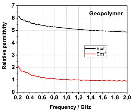
Fig. 10. Real part ( $\epsilon_{\text{r}}'$ ) and Imaginary part ( $\epsilon_{\text{r}}''$ ) of relative permittivity - Geopolymer
