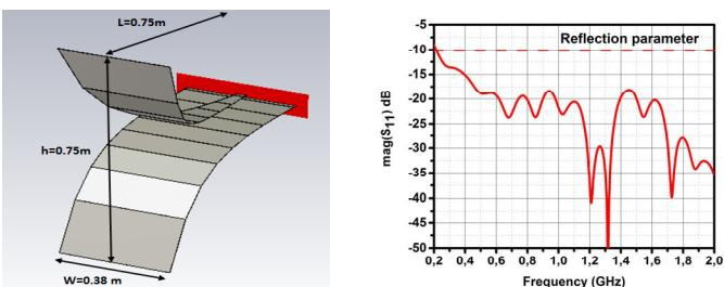
Fig. 3. Unbalanced Antenna and reflection coefficient magnitude
