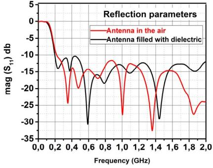
Fig. 6. Reflection coefficient magnitude
