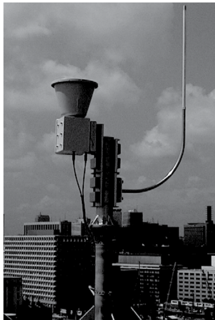
Figure 3.61 A base station antenna used in P-MP FWA systems [61].
