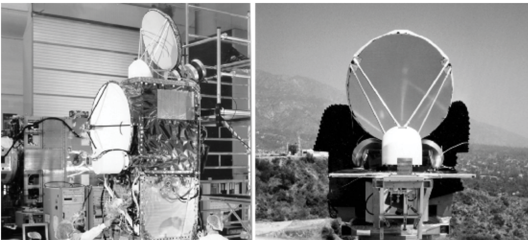
Figure 6.18 Jason 1 spacecraft is shown at left. The larger symmetric fed reflector is the altimeter antenna. The upper reflector is the radiometer, which is also shown in the photo at right.
