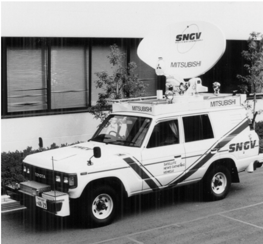
Figure 3.33 On-vehicle antenna mounted on the vehicle.
