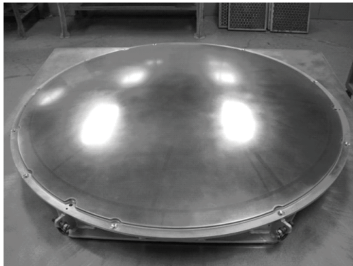
Figure 9.9 Invar reflector mold tool. (Copyright AASC 2012.)
