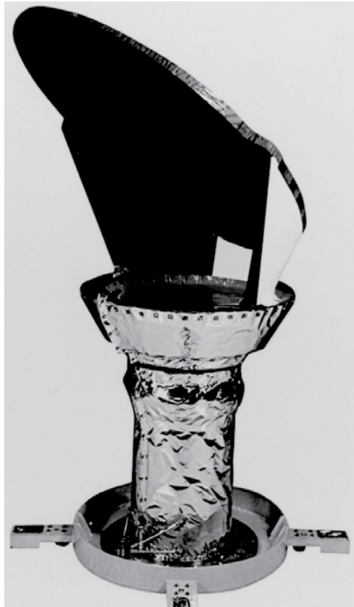
Figure 3.27 Photograph of the reflector assembly for CS-2 [28].
