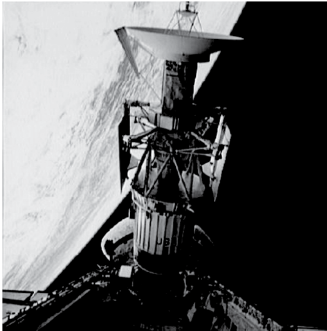
Figure 6.3 The Magellan spacecraft being deployed by the space shuttle Atlantis during STS-30 along with its inertial upper stage (IUS). To the left of the reflector antenna, the altimeter antenna (ALTA) instrument is also visible.
