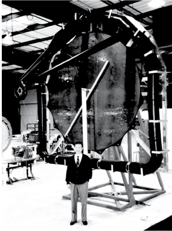
Figure 6.34 Three-meter Ka-band flat membrane inflatable reflectarray antenna.
