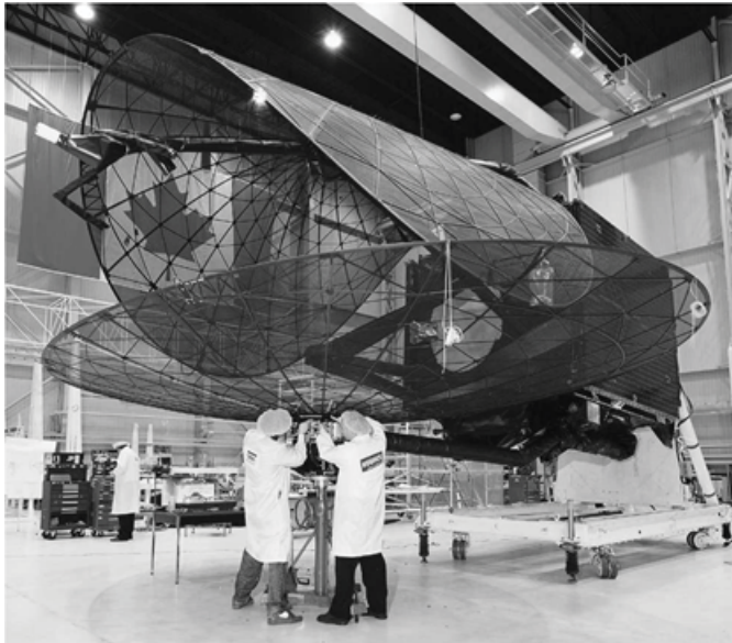
Figure 8.5 Hughes spring-back antenna: spacecraft with one reflector deployed and one partially stowed. (© 2002 IEEE. From [5].)
