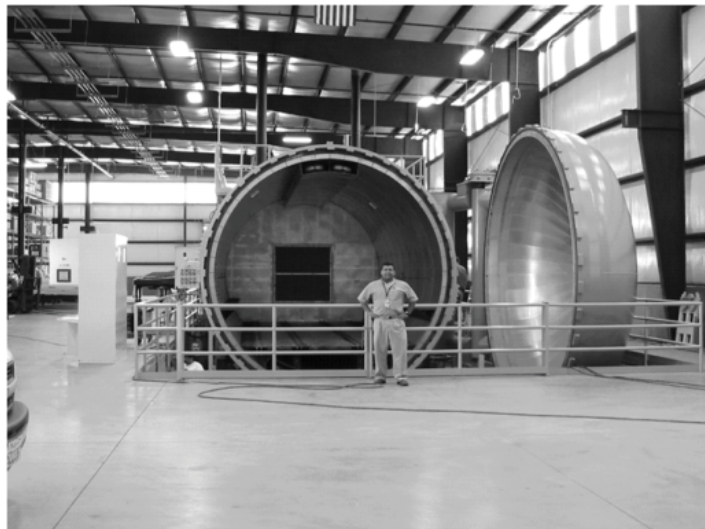
Figure 9.13 A 16-ft \times 30-ft autoclave. (Copyright AASC 2012.)
