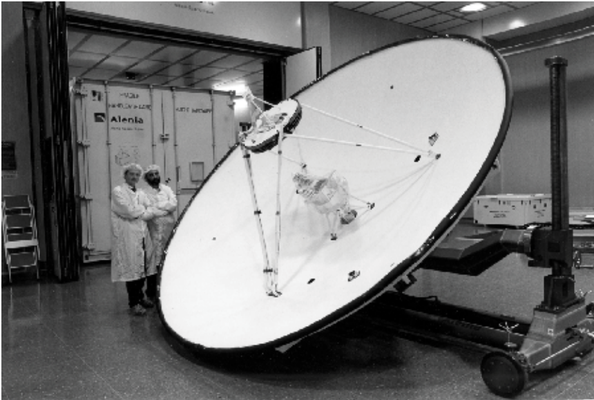
Figure 6.9 The complete Cassini antenna before being integrated with the spacecraft.
