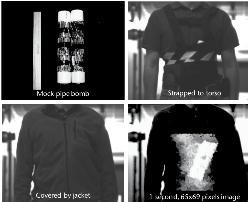
Figure 4.1 Photos showing through-clothes concealed weapon imaging with a 675- GHz FMCW radar at a 25m stand-off distance [11].
