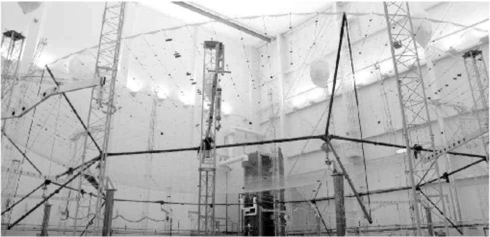
Figure 8.24 Harris hoop-truss reflector deployed (courtesy Harris Corporation).
