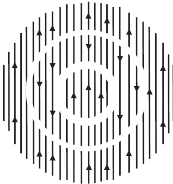
Figure 3.2 Vectorial representation of a paraboloid focal plane field, corresponding to Figure 3.1, including up to three nulls.
