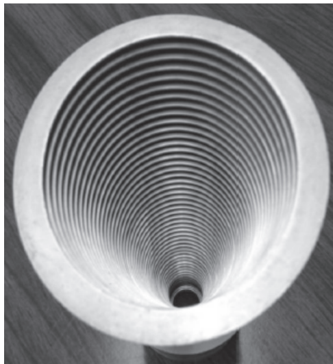
Figure 6.2 Photo of Ku-band elliptical corrugated feed horn for a Gregorian reflector antenna. Aperture aspect ratio is 1.2:1 [18].
