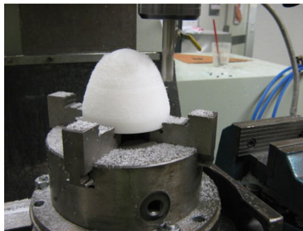
Fig. 28 Lens fabrication by CNC milling machine technique
