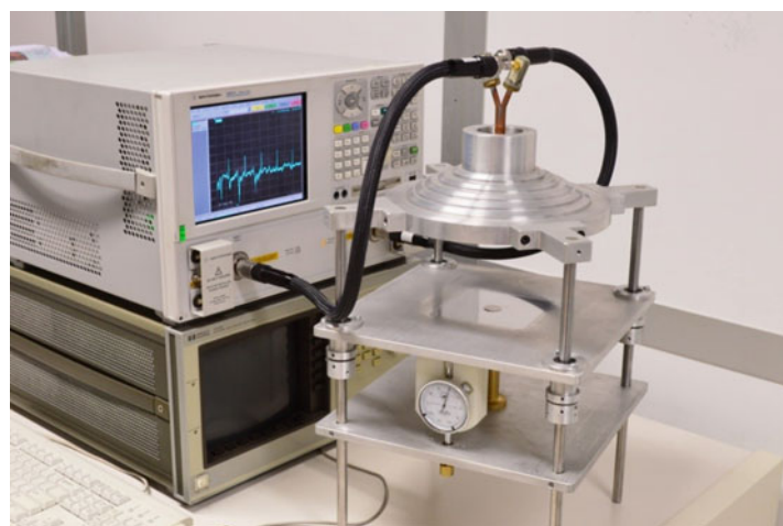
Fig. 27 Fabry-Perot open resonator for complex permittivity measurements in V-band
