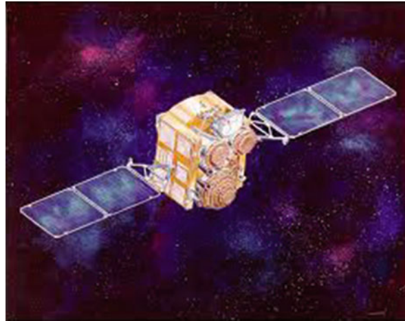
Fig. 14 Classical application of waveguide lens array antenna used in DSCS-III satellite
