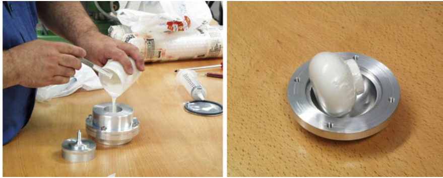
Fig. 29 Lens fabrication by molding technique
