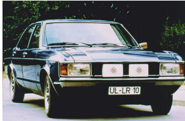
Fig. 1 Vehicle with a first 35 GHz radar (separate parabolic reflector antennas for transmit and receive, photograph TELEFUNKEN)
