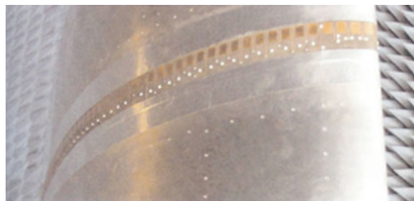
Fig. 67 An array of microstrip antennas are made conformal to a wing shape surface (Courtesy of Air Force Research Lab./ Antenna Technology Branch, Hanscom AFB, USA)
