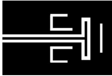
Fig. 20 Slotted quasi-Yagi-Uda feed as surface-wave launcher (similar to Podilchak et al. 2009)
