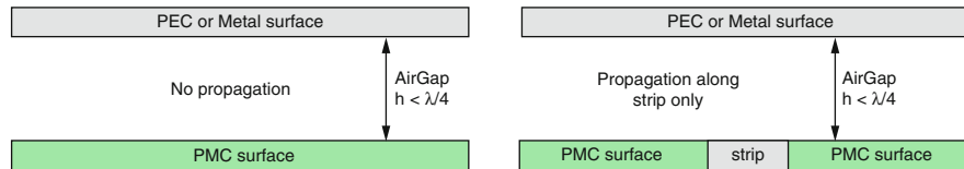
Fig. 1 Cross section of ideal gap waveguide (With permission from Zaman et al. 2014)
