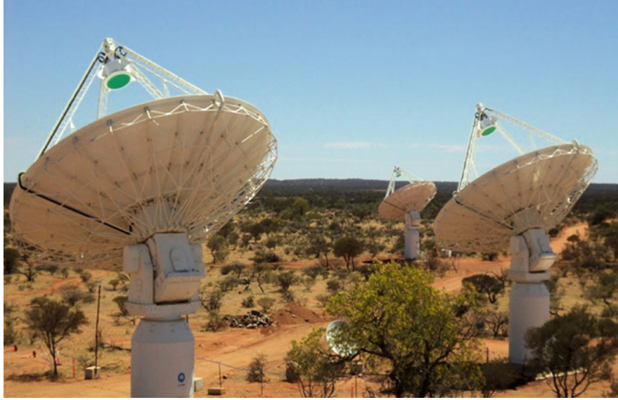
Fig. 35 Reflectors antennas in the Australian SKA pathfinder (ASKAP) (Courtesy CSIRO). This array consists of 36 12 m-diameter antennas, which are fed with 188 element phased array feeds, operate over a frequency range from 0.7 to 1.8 GHz (Picture courtesy CSIRO Australia)
