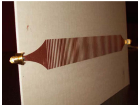
Fig. 16 Photograph of a 1-D leaky-wave antenna based on sinusoidally modulated reactance surface (Patel and Grbic 2011, © IEEE)
