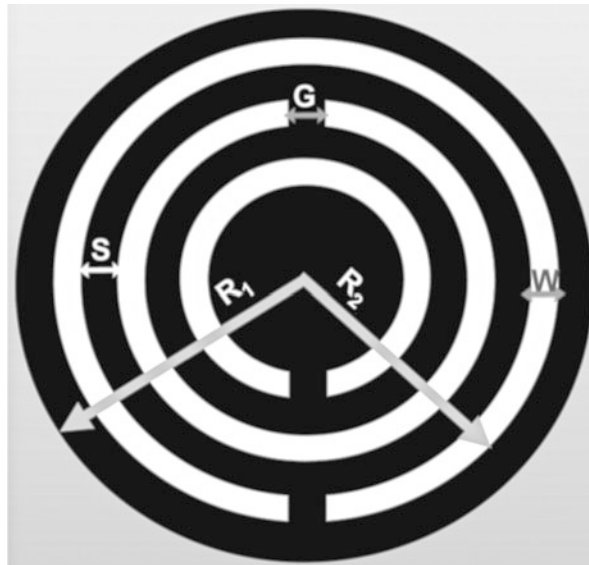
Fig. 42 Geometry of the disk containing CSRR (© IEEE 2015)
