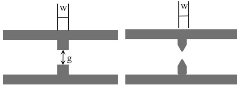
Fig. 6 The geometry of photoconductive antennas common dipole and sharp dipole
