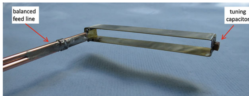
Fig. 10 Directly tapping across a loop using a balanced feed. The balanced line consists of two 50\ \Omega coaxial semirigid cables soldered together. The inners of the cables are fed from a 3 dB 180^\circ splitter that converts an unbalanced 50\ \Omega feed into two 50\ \Omega signals that are 180^\circ out of phase with each other, giving a balanced impedance of 50 + 50 = 100\ \Omega . To enable easy connection and disconnection between line and antenna, some sockets have been soldered onto the antenna, and wires which fit into the sockets have been soldered to the ends of the inner conductors of the coaxial cables. This arrangement is used for measuring the performance of different shapes of loops and for measuring the effects of bringing components close to the loop. The single adjustable tuning capacitor gives a very large tuning range but is very sensitive. For mass production, tuning using fixed capacitors in parallel with an adjustable capacitor is preferred. See Fig. 9
