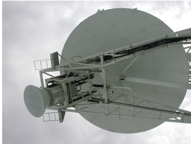
Fig. 2 GBT subreflector and prime focus feed. In this image, the prime focus feed is deployed (Image credit: B. Saxton, NRAO/AUI/NSF)
