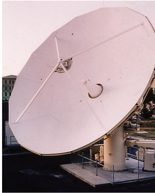
Fig. 30 An 11 m X-band earth station antenna that was designed for low profile and high isolation so as to meet the CCIR sidelobe specifications (Bird et al. 1995)
