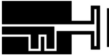
Fig. 15 Planar quasi-Yagi-Uda surface-wave launcher with balun as slot-line-to-coplanar waveguide transition
