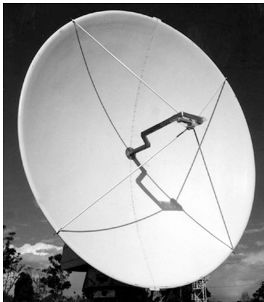
Fig. 34 A paraboloid reflector with high performance dual – polarized feed for a radar application (Hayman et al. 1998)
