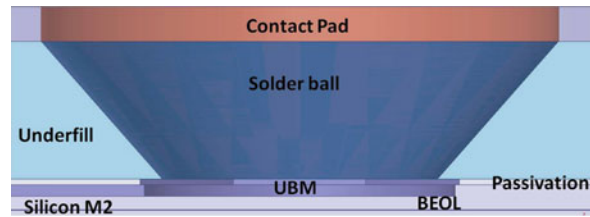
Fig. 17 Layer view of the flip-chip solder ball transition
