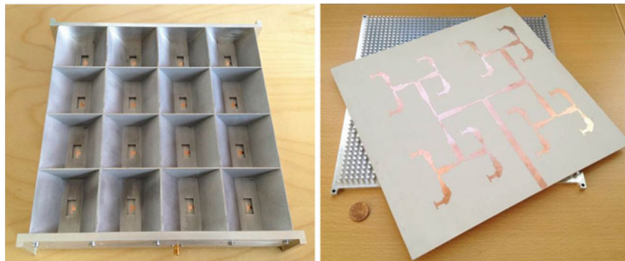
Fig. 33 Manufactured horn array with inverted microstrip gap waveguide feed network
