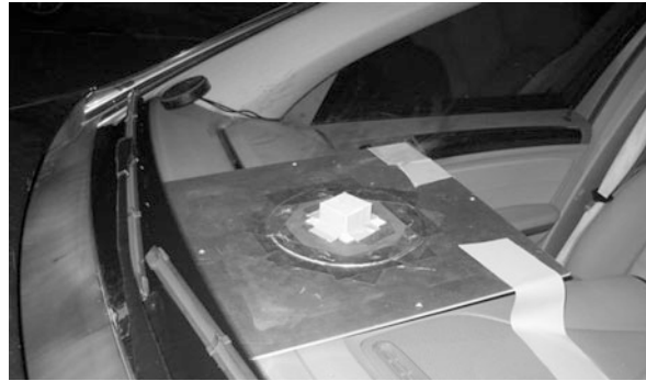
Fig. 41 Diversity antenna function demonstrator in a mounting volume of 29 \times 29 \times 11 \text{ mm}^3 on dashboard of a test car
