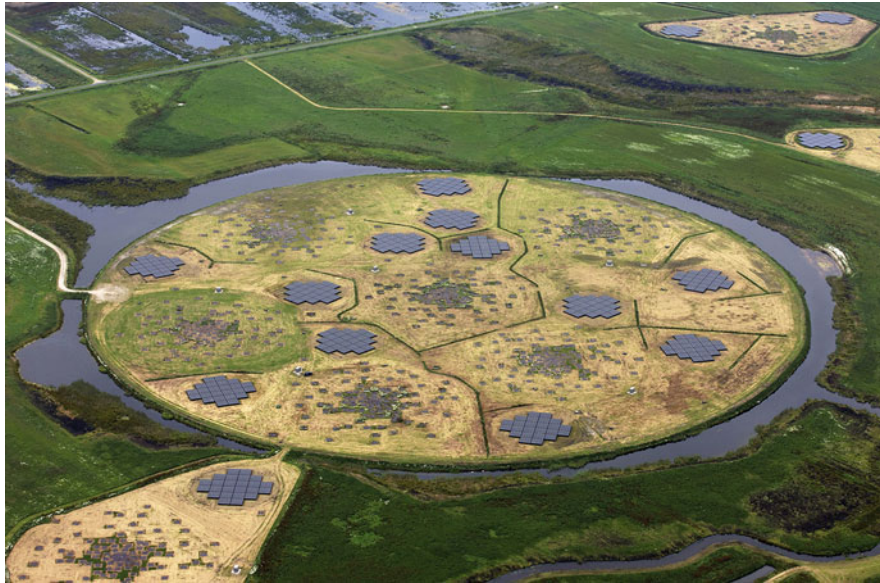
Fig. 12 An aerial view of the LOFAR “superterp,” a region within the 2-km-diameter “core” region, within which 24 of the stations are located. Nine stations are visible here: 6 within the circular island in the center of the image, one at the lower left , and two more on the upper right . The square dark-colored panels are HBA tiles, organized here into 24-tile subarrays. The smaller dark-colored patches are the ground screens of individual LBA antennas (Credit: van Haarlem et al. (2013) A&A, 556: A2, reproduced with permission © ESO)
