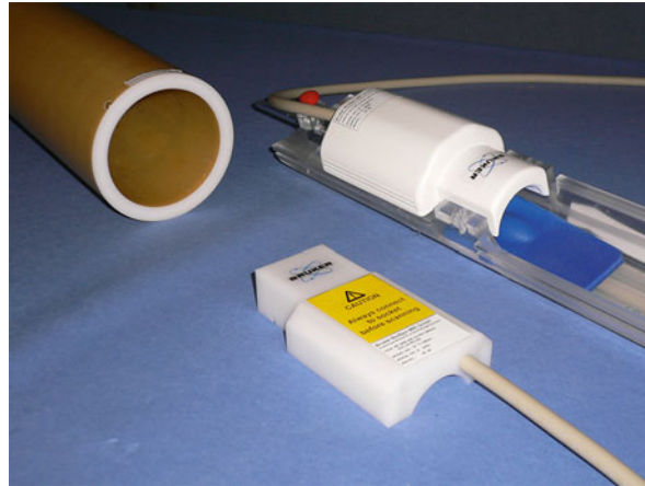
Fig. 1 A Set of RF coils for preclinical imaging of small objects consists of a volume coil for RF transmission and a two local RF coils for MRI signal detection
