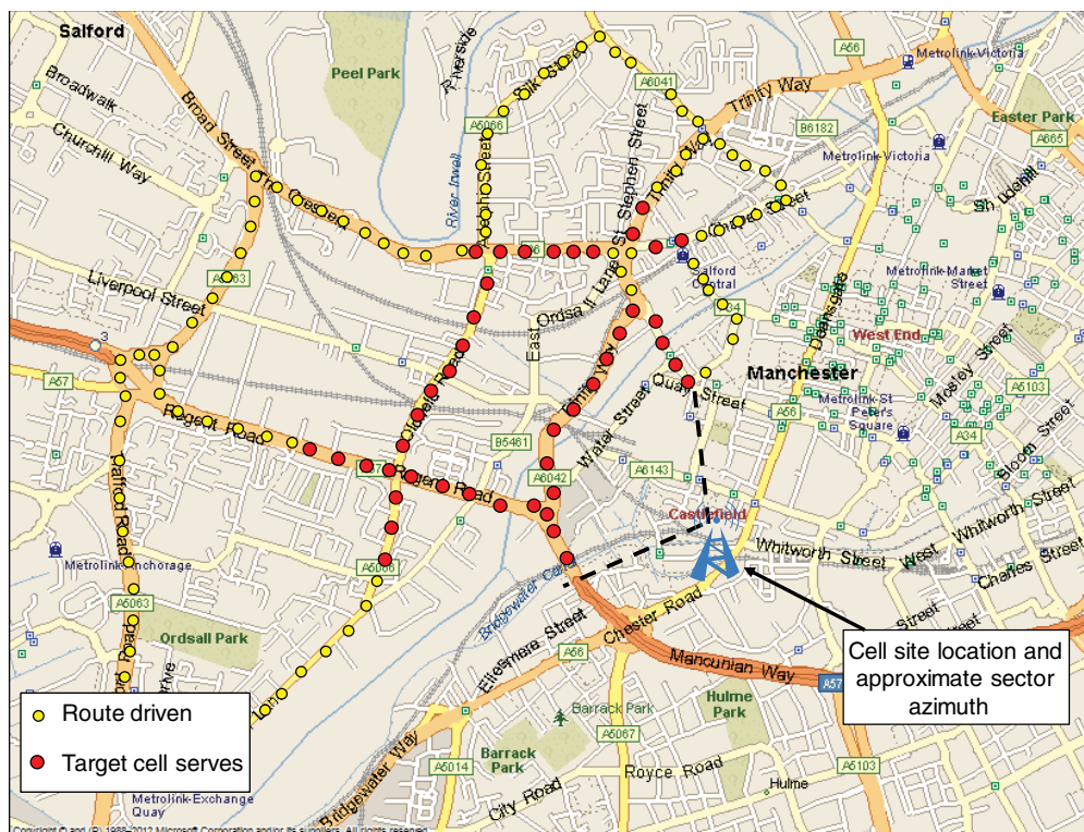
Figure 7.14 Cell coverage surveys: outline survey. Source: Microsoft AutoRoute map reproduced with permission from Microsoft
