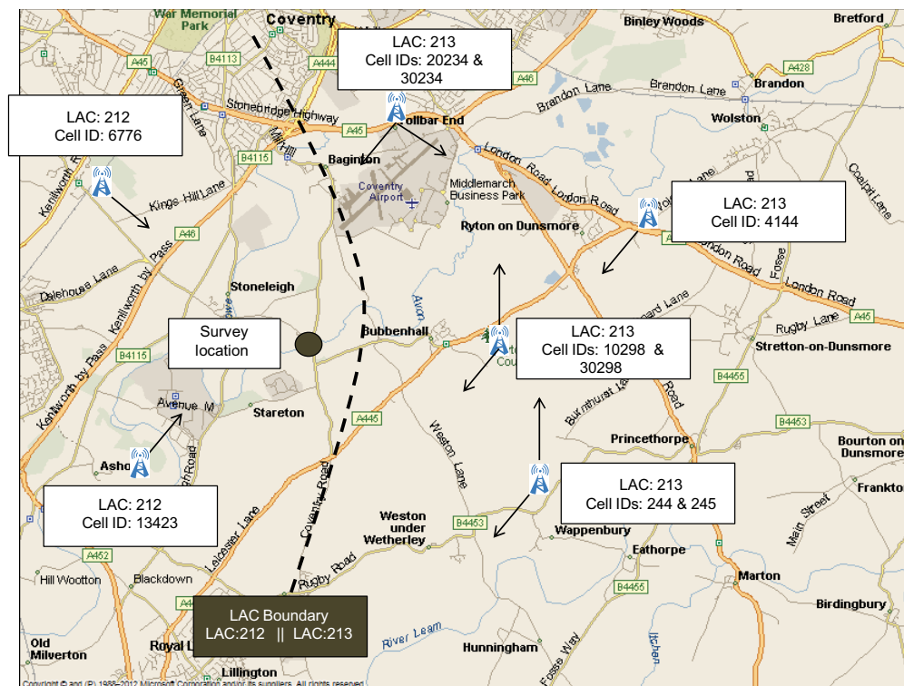
Figure 7.17 Surveying near a LAC boundary. Source: Microsoft AutoRoute map reproduced with permission from Microsoft
