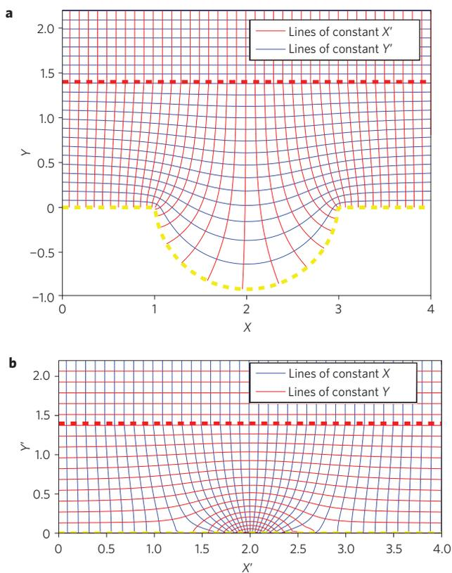
**Figure 2 | The transformation used to produce the flattened Luneburg lens.** The material used to realize the flattened Luneburg was designed with a numerically generated quasi-conformal spatial transformation. **a,b**, The resulting map (**a**) and its inverse (**b**). Materials designed in this manner are inherently broadband, as they require only dielectric materials.
