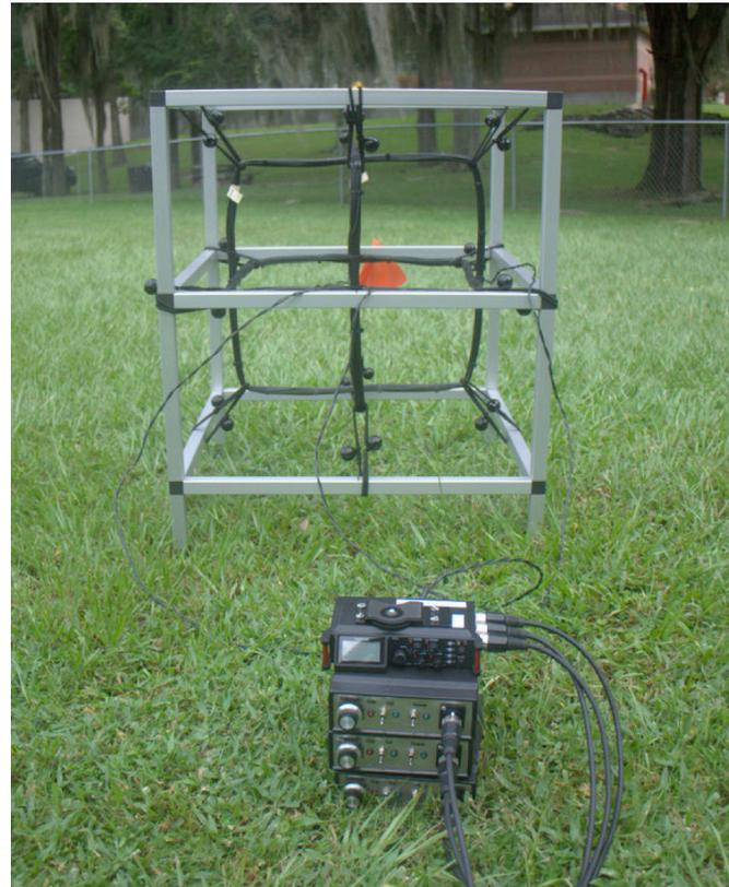
Fig. 2. The portable 3-axis magnetic field receiver.
