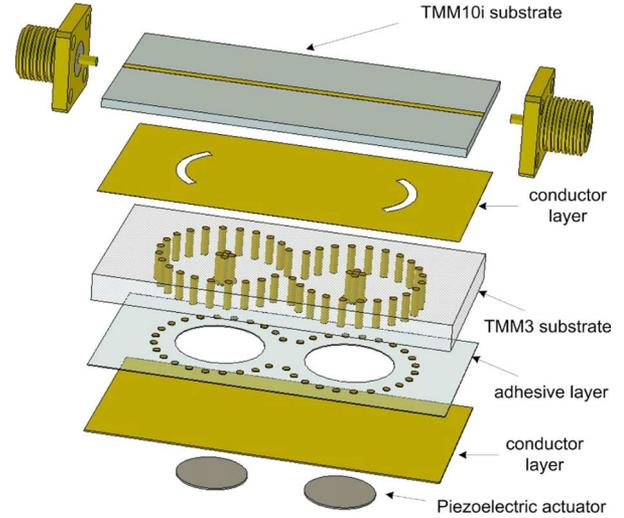
Fig. 2. Proposed bandstop filter with two substrated-integrated evanescent-mode cavity resonators.
