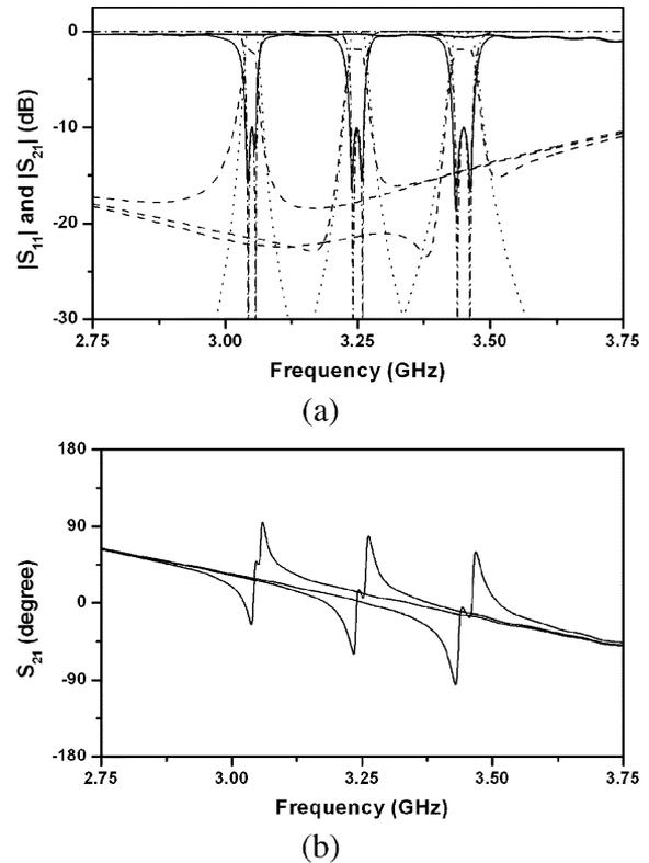
Fig. 4. Measured frequency response of the fabricated bandstop filter. The filter is tuned to exhibit Chebyshev bandstop responses with 10 dB stopband rejection at three different center frequencies: (a)  $|S_{11}|$  measurement (—),  $|S_{21}|$  measurement (—),  $|S_{11}|$  synthesis ( $\cdot \cdot \cdot$ ),  $|S_{21}|$  synthesis (— · —), (b)  $S_{21}$  (degree) measurement.
