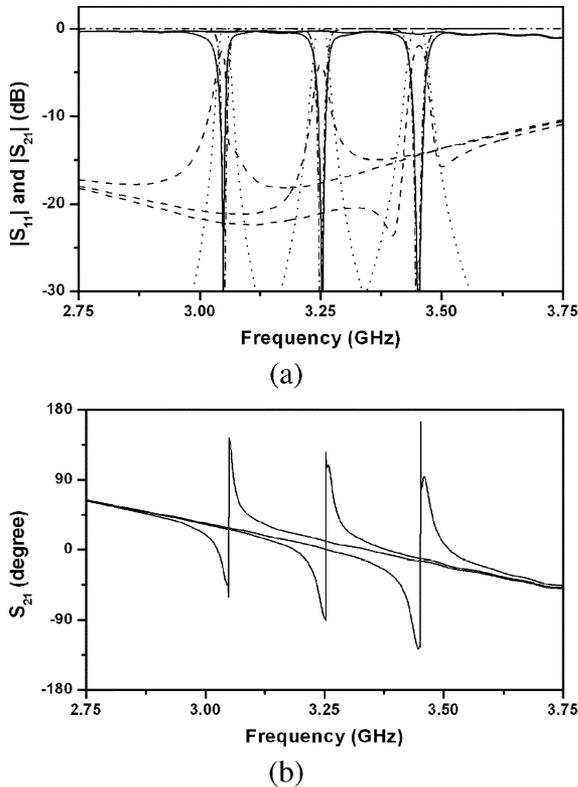
Fig. 3. Measured frequency response of the fabricated bandstop filter. The filter is tuned to exhibit Butterworth bandstop responses at three different center frequencies: (a)  $|S_{11}|$  measurement (—),  $|S_{21}|$  measurement (—),  $|S_{11}|$  synthesis ( $\cdot \cdot \cdot$ ),  $|S_{21}|$  synthesis (— · —), (b)  $S_{21}$  (degree) measurement.
