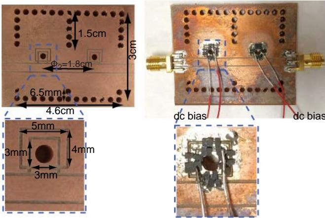
Fig. 4. Fabricated two-pole band stop filter (a) without the surface mount diodes and (b) with the surface mount diodes.
