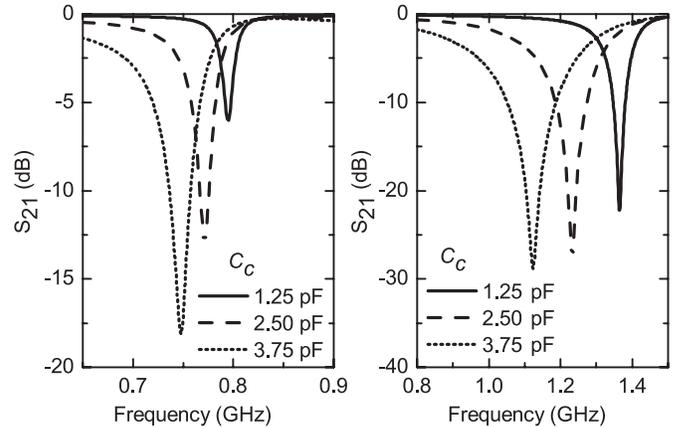
Fig. 3. Simulation from HFSS shows tunable bandwidth at the (a) lower tunable frequency and at the (b) higher tunable frequency.
