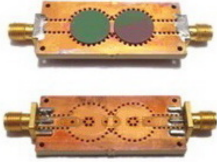
Fig. 4. Fabricated prototype of the proposed bandpass filter a) top view b) bottom view.
