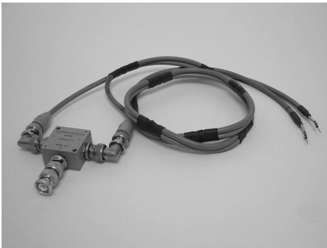
FIGURE 18-9. A home-made X10, passive, differential voltage probe, with a 180° combiner.
