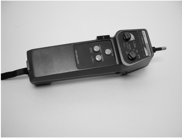
FIGURE 18-28. A small battery powered ESD simulator.
