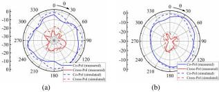
Fig. 4 Measured co-polarization and cross-polarization patterns at 3.56 GHz
