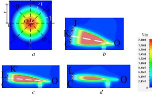
Fig. 1 Simulated magnitude of electric field distribution a Circular SIW cavity b sixteenth mode SIW (SMSIW) c thirty-second mode SIW (TMSIW) d SFMSIW
