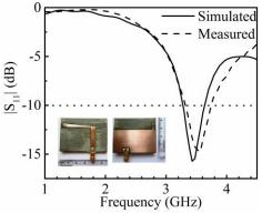
Fig. 3 Simulated and measured reflection coefficients of the proposed antenna (antenna front and back have been shown in inset)
