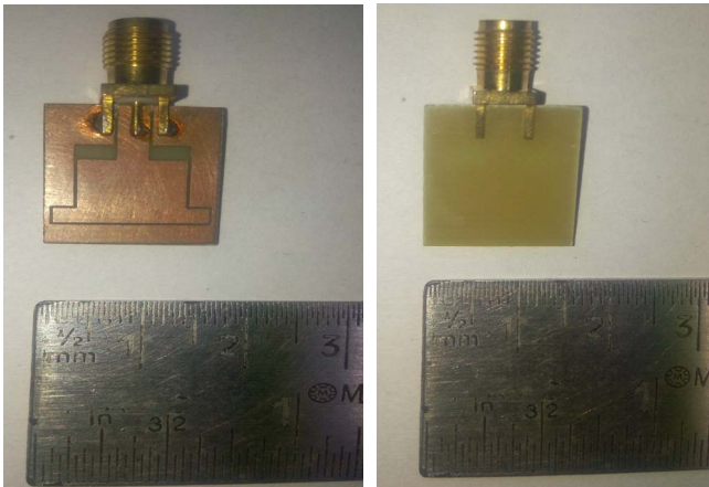
Fig. 6. Fabricated prototype of the presented CPW-fed ZOR antenna.
