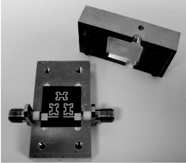
Figure 5.20 Third-order meandered line pseudo-elliptic filter with a transmission zero on the right.
