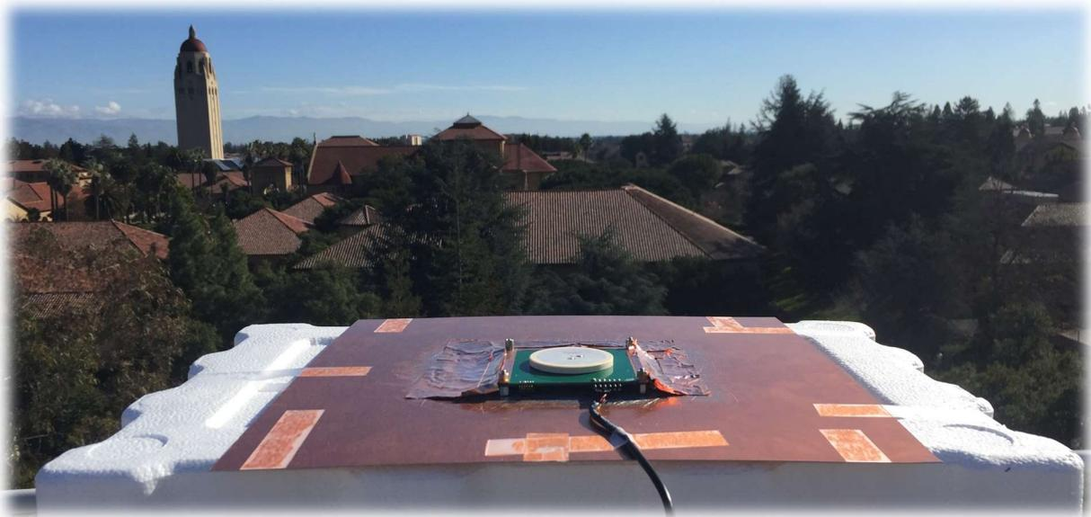
Figure 6. Static testing at Stanford rooftop with flat ground plane
