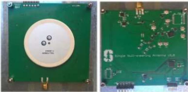
Figure 2. Stanford PCB Dual Polarization Antenna
