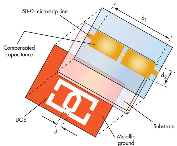
3. This is a three-dimensional (3D) view of the DGS bandstop filter (BSF).
