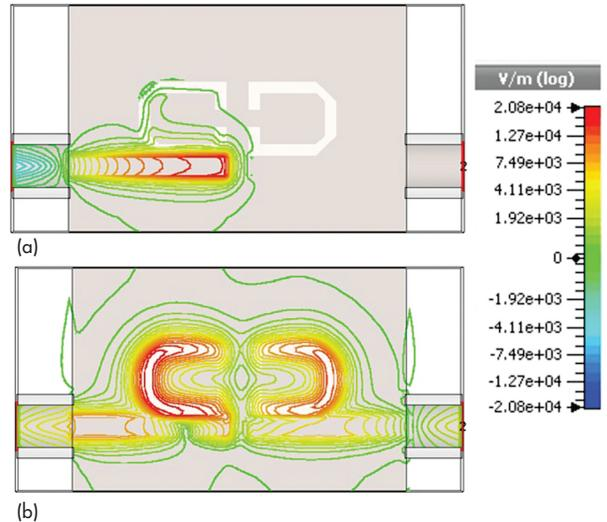
13. These are electric-field distribution results for the BPF: (a) in the stopband at 3.5 GHz and (b) in the passband at 4.8 GHz.
