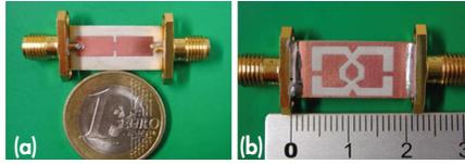
4. These photographs show the fabricated DGS BSF: (a) top and (b) bottom.
