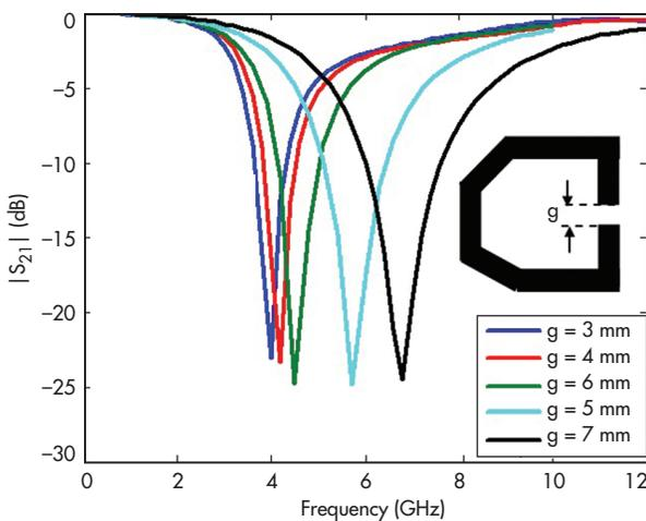
2. These simulations of  $S_{21}$  insertion loss show the impact of changing gap width  $g$ .
