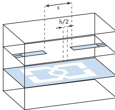
6. This is a 3D view of the DGS BPF formed from the use of a J-inverter with the BSF.
