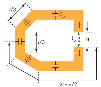
1. This represents a proposed DGS resonator and its equivalent-circuit model.
