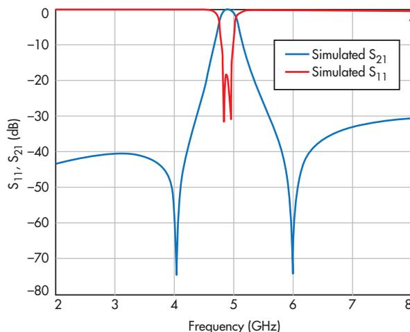
11. The traces show simulated S-parameters for the BPF.
