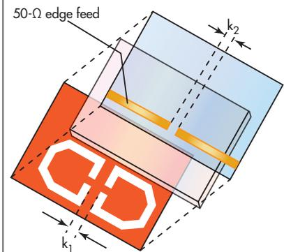
9. This is a 3D view of the DGS BF (with the feeds on the edges).
