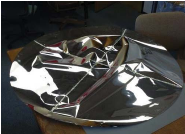
Figure 6.8 Inflatable antenna manufacturing and petals bonding on the reflective side [16]. Reproduced with permission of IEEE.
