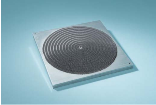
Figure 8.29 Fabricated 20 cm diameter Ka-band metal-only antenna.
