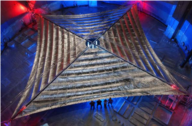
Figure 1.8 NeaScout solar sail fully deployed. Courtesy of NASA.
