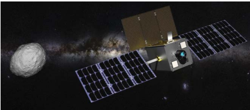
Figure 5.3 ESA's 12U CubeSat M-Argo using a deployable reflectarray antenna [7]. Courtesy of European Space Agency.
