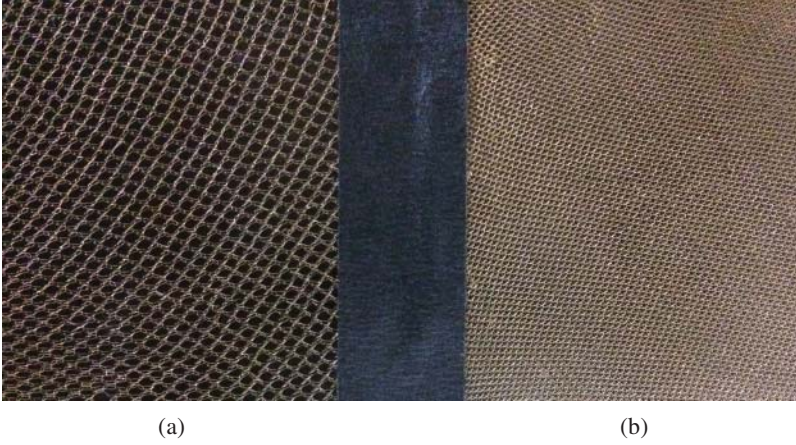
Figure 3.29 Photography of two mesh with different OPI: (a) 40-OPI mesh; (b) 10-OPI mesh.
