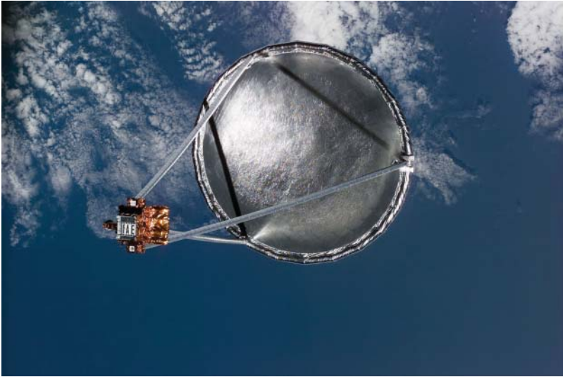
Figure 6.4 Inflatable antenna experiment on board the STS-77. Credits: NASA [9].
