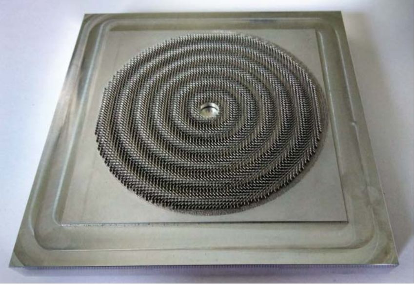
Figure 8.3 Ka-band modulated metasurface antenna fabricated by metal additive manufacturing [32].
