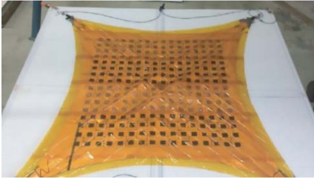
Figure 1.26 S-band 1.5\text{ m}^2 aperture deployable membrane antenna after its first deployment [22].
