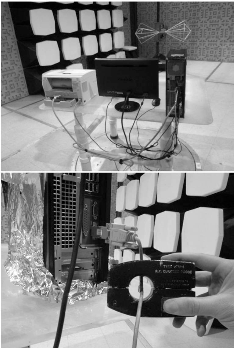
Fig. 13.7 Example of EMI investigation routine on a computer, installed for radiated emission testing ( top ). After failing the Class B limit, the CM current is checked on the CPU data cable. As a variation of the routine steps, the unit is tightly wrapped in aluminum foil, in order to prevent box leakages from obscuring our diagnosis (photos courtesy of Don Sweeney, D.L.S. Electronic Systems Inc.)
