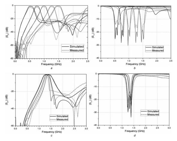
Fig. 6 Measured and simulated results of centre frequency tunability of Design #1
