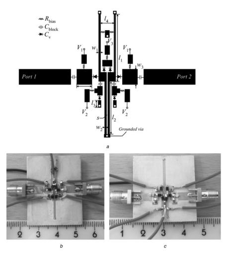
Fig. 5 Configuration of the proposed tunable BPF
