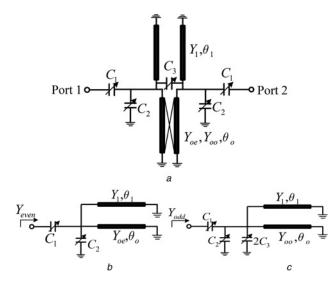
**Fig. 1** Schematic diagram of the proposed tunable BPF *a* Transmission line schematic of the proposed filter *b* Even-mode equivalent circuit *c* Odd-mode equivalent circuit
