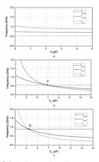
**Fig. 2** Relation between resonant frequencies  $(f_{even}, f_{odd})$ , transmission zero  $(f_{tz1})$  and the capacitances
