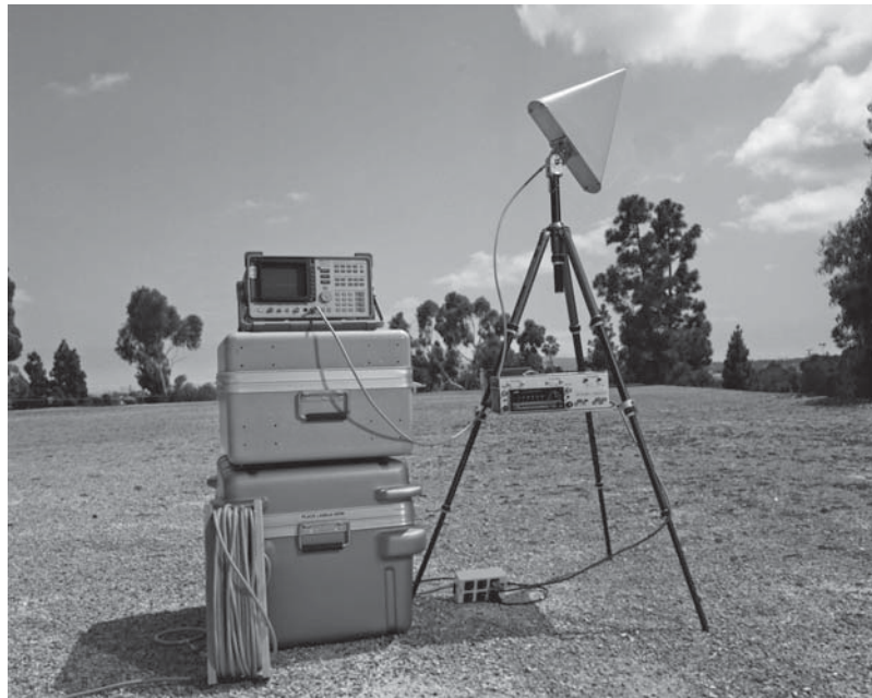
Figure 5-2 RF site survey equipment [1]
