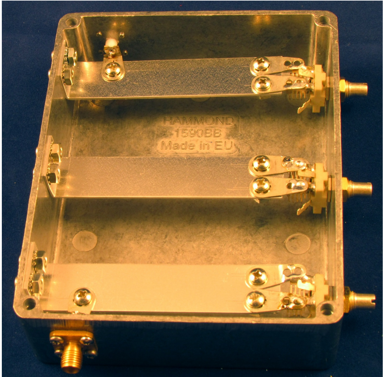
Figure 8 – Combine filter for 432 MHz in diecast box
