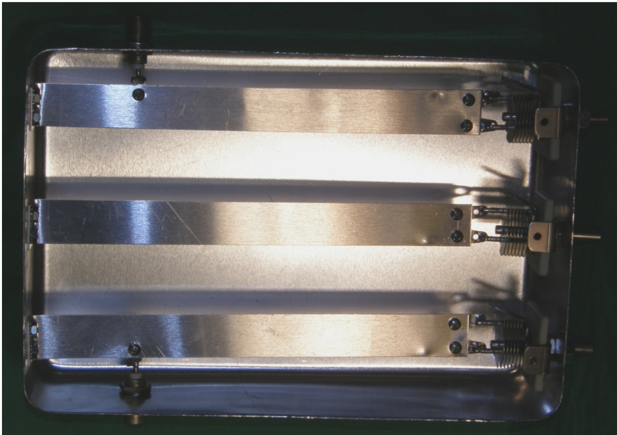
Figure 2 – Compline Filter for 144 MHz
