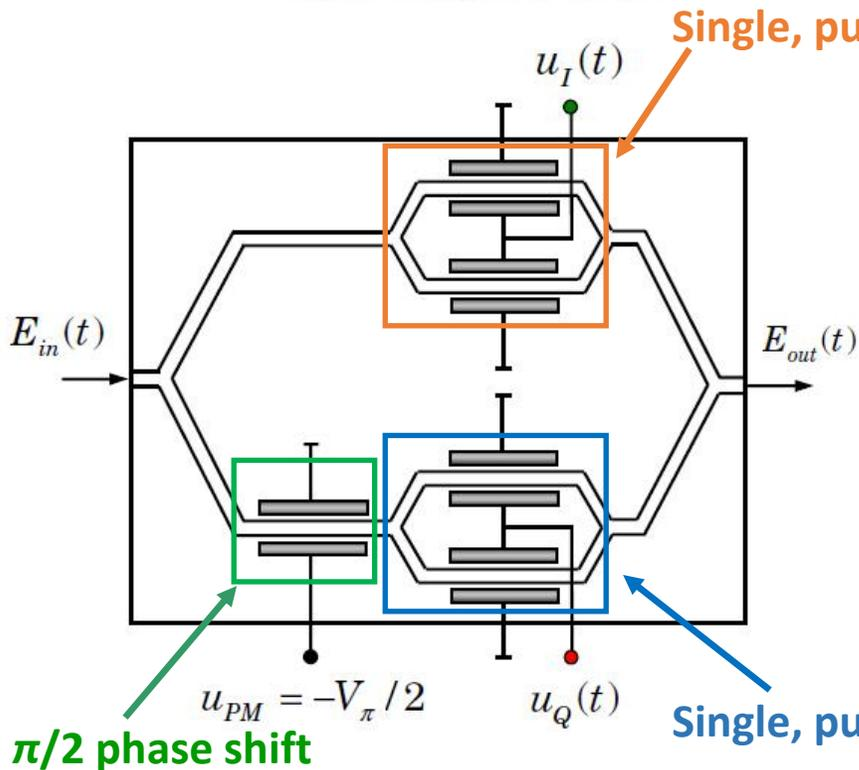
Single, push-pull MZM modulating the In-Phase component
