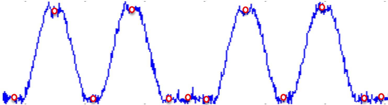
After sampling time correction, we obtain samples at the optimum points (the middle of the pulses)
