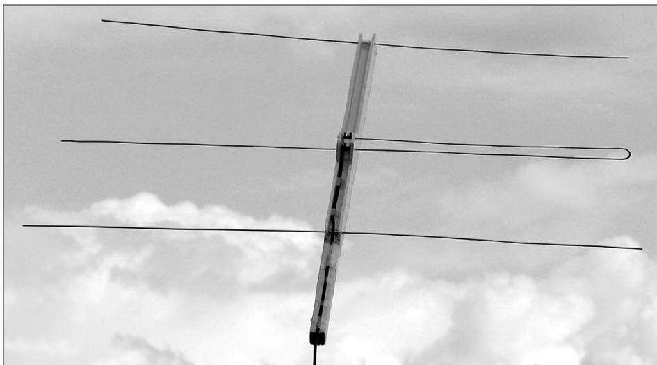
Photo 1: The N2SPI Cheap and Easy Satellite Uplink Antenna.
