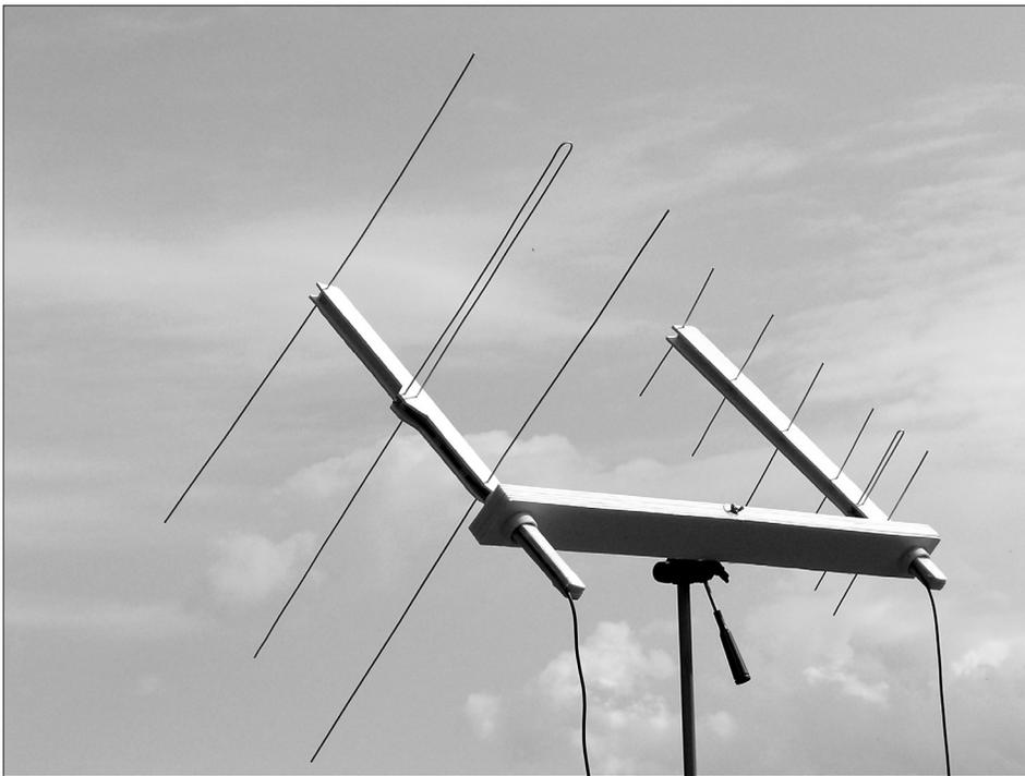
**Photo 5: Uplink antenna, cross boom and downlink antenna, ready for AMSAT's AO-51 Echo satellite.**
