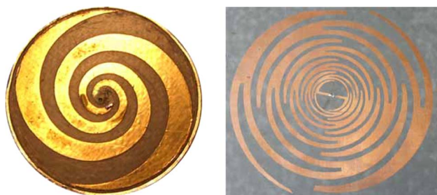
Fig. 13. Self-complementary antennas. (Left) Two-arm logarithmic spiral antenna and (right) sinuous antenna.
