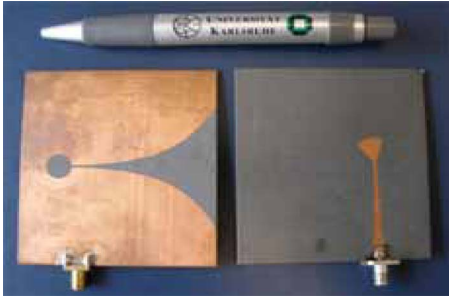
Fig. 6. Aperture coupled Vivaldi antenna. (Left) Top view; (right) bottom view with feed line. Substrate size 75 \times 78 \text{ mm}^2 .
