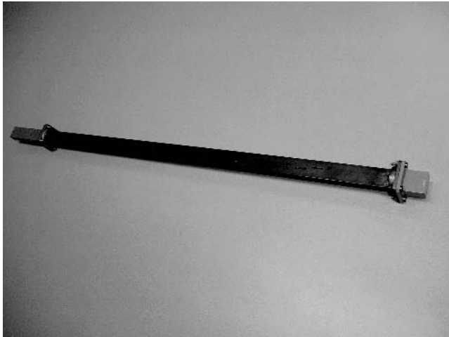
Fig. 8.8 Realised 21-slots slotted waveguide array antenna in WR90 having a coaxial to rectangular waveguide adapter connected to one side and a waveguide load to the other side.
