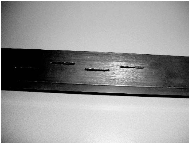
Fig. 8.12 Detail of the slotted waveguide array antenna of figure 8.8.
