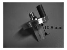
FIGURE 38-4 Fabricated resistively loaded monopole antenna soldered to an SMA connector and attached to a metal plug (after J. M. Sill and E. C. Fear<sup>43</sup> © IEEE 2005)
