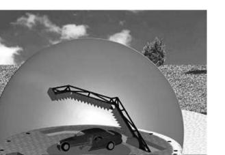
FIGURE 39-34 Outdoor near-field antenna facility with radome (*Courtesy of Hirschmann Car Communication, Inc.*)
