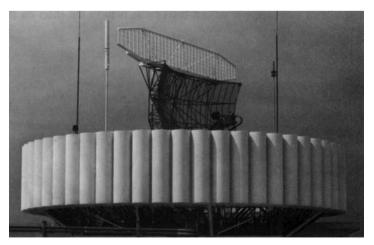
FIGURE 43-18 E-SCAN cylindrical array (Courtesy of Hazeltine Corporation)
