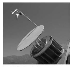
FIGURE 35-20 X/Ka dual-band Cassegrain reflectarray antenna (0.75-m diameter) using annular ring elements
