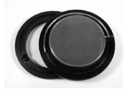
FIGURE 38-11 Circumference antenna on a pacemaker model (after A. Johansson, <sup>169</sup> Figure 5-3)
