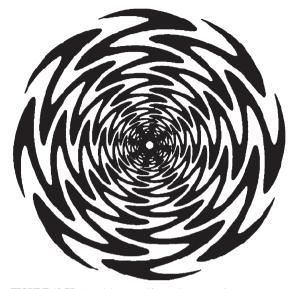
FIGURE 13-75 An eight-arm self-complementary sinuous antenna
