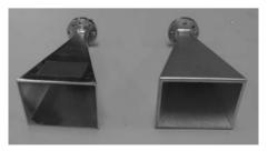
FIGURE 23-4 Horn antennas, connected to a WR15 waveguide, operating at millimeter-wave frequencies. The horn antenna on the left is precision assembled whereas the horn on the right is cast and plated for lower cost.
