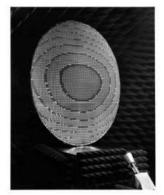
FIGURE 35-18 Ku-band reflectarray with shaped contour beam capability (*Courtesy of Professor Dave Pozar, Univ. of Massachusetts*)
