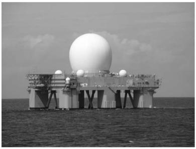
(b) Radomes for sea-based radar and communication antennas
