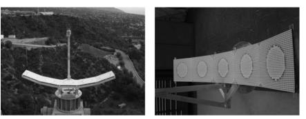
FIGURE 35-24 Piece-wise flat reflectarray for space application
