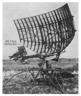
**FIGURE 43-13** Tactical S-band radar antenna with integral IFF feed (*Courtesy of Thomson-CSF*)
