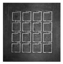
FIGURE 31-9 Photograph of a 4×4 array of pattern reconfigurable elements that can be configured to deliver broadside, endfire, and scanned radiation patterns (after G. H. Huff<sup>18</sup> © 2006)
