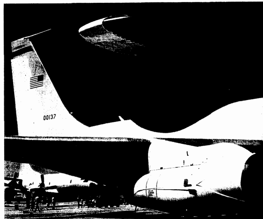
FIG. 32-6 AWACS antenna in rotodome mounted on the tail section of a Boeing 707-320 aircraft.
