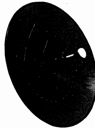
FIG. 33-21 IFF array for airborne fire-control radar. (Courtesy Hazeltine Corporation.)
