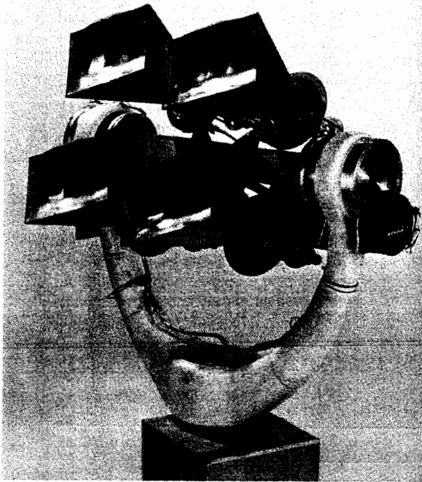
FIG. 40-7a Four-horn sequential-lobing tracking antenna (1 to 5 GHz).
