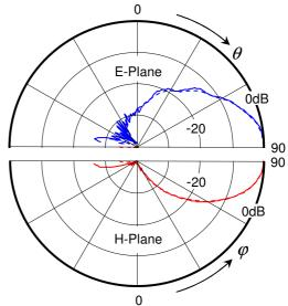
Fig. 5. Comparison of measured and calculated radiation patterns, E-Plane (upper) and H-plane (lower) at 10GHz.
