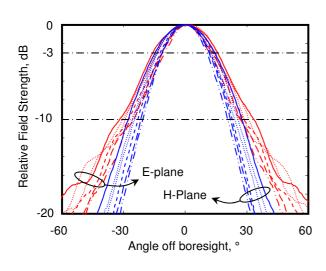
Fig. 4. Expanded radiation pattern, both E- and H-Planes, 8-13GHz
