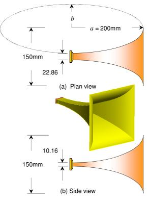
Fig. 1. Plan (a) and side (b) views of the elliptic horn
