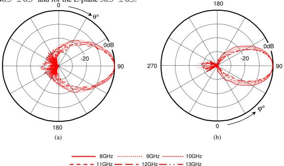
Fig. 5 compares the calculated and measured radiation patterns for both principal planes at 10GHz; for all practical purposes calculated and measured patterns are identical.
