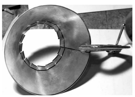
Figure 15 — Bend the flange into a circle, holding with vise grips, solder the seam.
