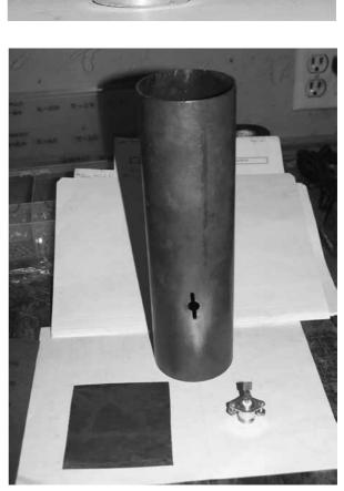
Figure 9 — Materials ready for assembly. The cut cylinder, copper plate for closing the end of the pipe, and the probe assembly.
