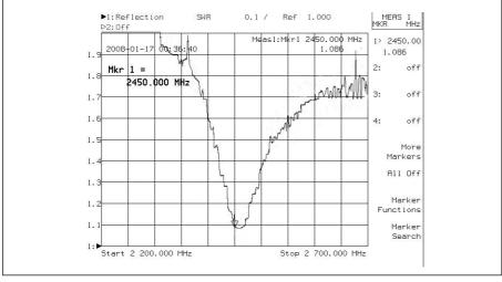
Figure 20 — Actual screen shot of SWR bandwidth boasting 1.086 at 2.45 GHz.
