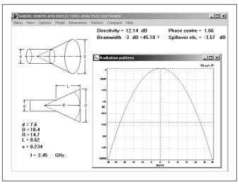
Figure 22 — SABOR X-Y Plot of the pattern. Gain is 12.14 db and the 3 db beam width is 45 degrees.
