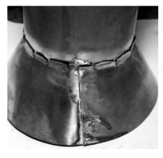
Figure 16 — Cylinder with flange fitted over pipe ready to solder. This may take quite a bit of heat.
