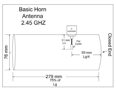
Figure 5 — Basic Horn Antenna Design.
