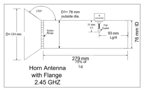
Figure 17 - Diagram of Complete Hooded Horn antenna.
