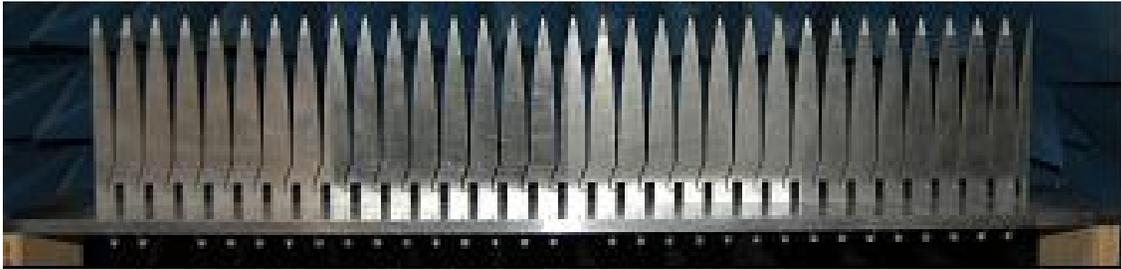
Fig. 2. 32-element linear array of flared notches. The array is constructed from modular sub-arrays of 8 elements.
