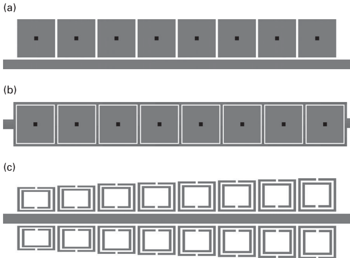
Figure 5.20 Comparison of the eighth-order filter based on the GPR and filter based on SRR: (a) Filter with GPR resonator placed next to microstrip line. (b) Filter with patch resonators implemented in microstrip line. (c) Filter based on SRRs [18].
