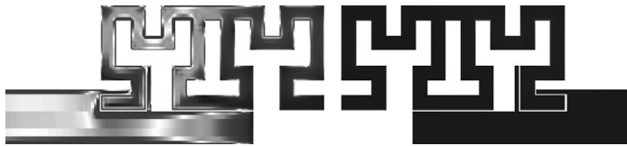
Figure 6.17 Current distribution at the frequency of transmission zero.
