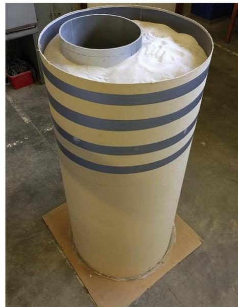
Fig. 14. Laboratory column consisting of an outer paper tube, inner plastic tube and dry sand between both tubes (see Fig. 13).
