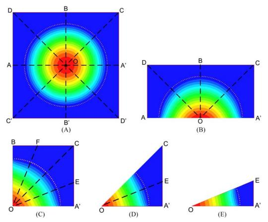
**FIGURE 1** Simulated electric field distributions: (A) Full-mode SIW; (B) Half-mode SIW (HMSIW); (C) Quarter-mode SIW (QMSIW); (D) Eighth-mode SIW (EMSIW); (E) Sixteenth-mode SIW (SMSIW). [Color figure can be viewed at wileyonlinelibrary.com]
