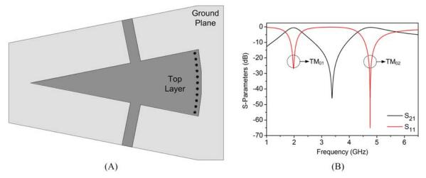
FIGURE 3 (A) Single cavity structure; (B) Simulated frequency response. [Color figure can be viewed at wileyonlinelibrary.com]
