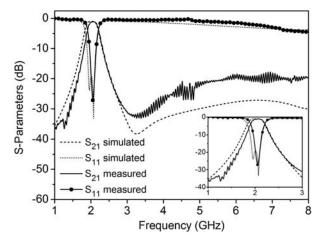
FIGURE 10 Simulated and measured filter response
