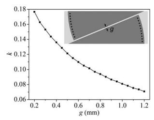
FIGURE 7 Coupling coefficient against g
