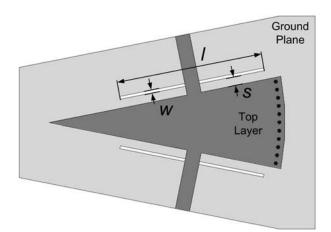
FIGURE 4 Single cavity with ground slots
