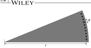
FIGURE 2 Configuration of SMSIW circular cavity
