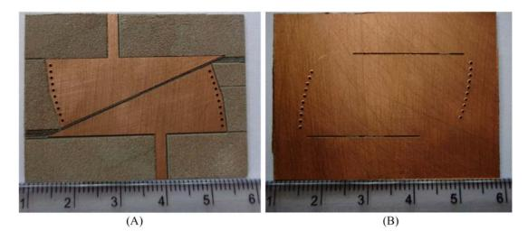
FIGURE 9 Photograph of fabricated filter: (A) Top view; (B) Bottom view. [Color figure can be viewed at wileyonlinelibrary.com]
