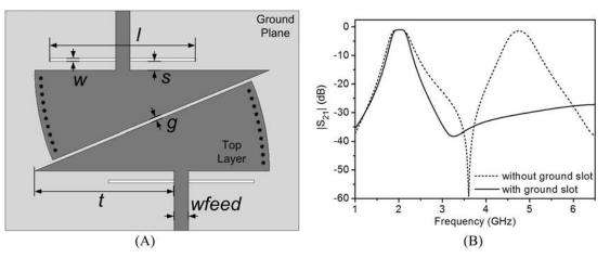
**FIGURE 8** (A) Two-pole bandpass filter with slots on ground plane; (B) Comparison of  $|S_{21}|$  (dB) of bandpass filters with and without slots on ground plane
