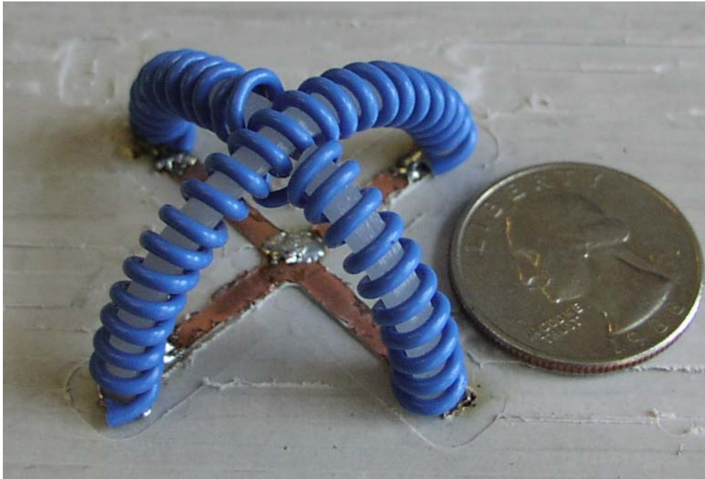
Figure 6: A photograph of the constructed antenna.
