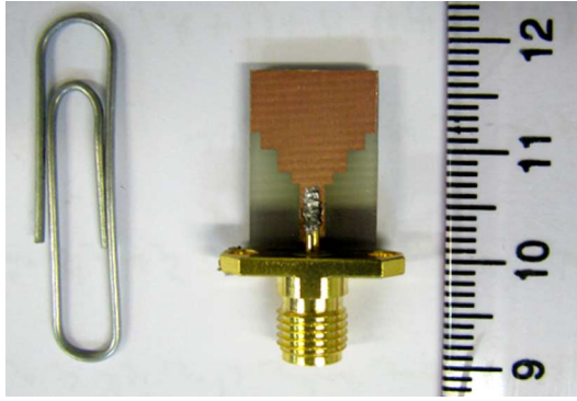
Fig. 5. Photograph of the realized compact monopole antenna.
