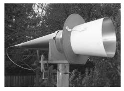
Here is a completed 144 MHz launcher, mounted to a wooden frame for testing.
