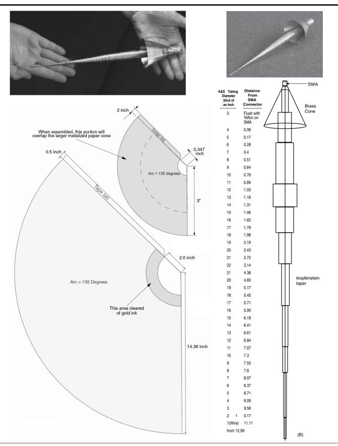
Figure 2 — Part A shows the metalized paper and brass shim stock cone patterns before folding. Part B gives the dimensions of the inner launcher tapered conductor sections made from K&S Metals brass tubing (in 32nds of an inch) versus position from the SMA connector for the 400 MHz launcher.
