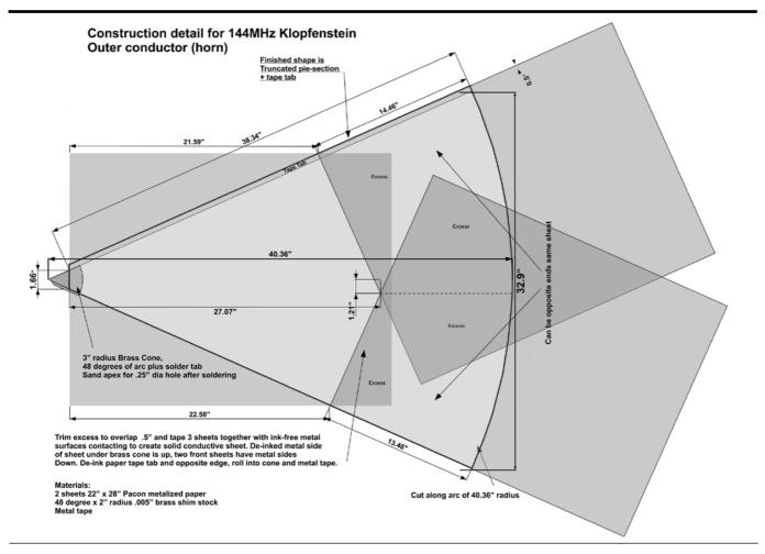
Figure 4 — The paper cone for the 144 MHz version of the launcher requires three 18 × 24 inch sheets of metalized paper.
