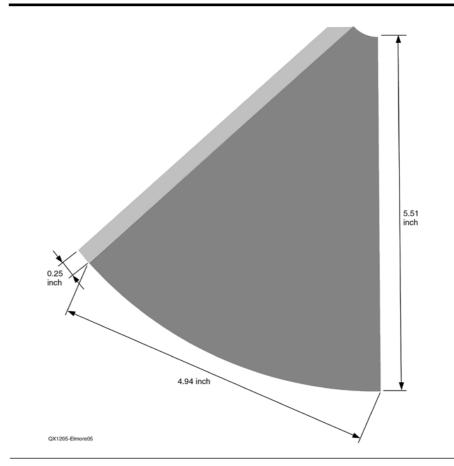
Figure 5 — This is the template for the brass portion of a 144 MHz launcher outer cone. The material can be 0.01 inch thick brass shim stock.
