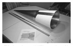
This photo shows a 144 MHz cone, along with the Klopfenstein taper impedance matching line and the template sheet for the cone.
