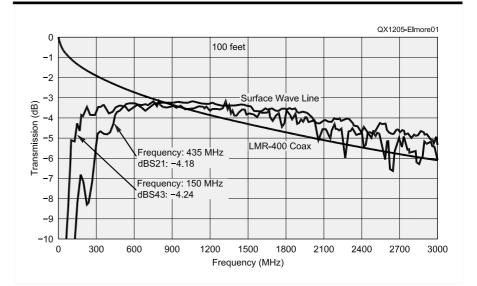
Figure 1 — Measured performance of SWTL compared with measurement of Times Microwave LMR-400 coaxial cable. Plots of 100 feet of no. 24 AWG conductor with a pair of 400 MHz launchers and a pair of 144 MHz launchers are shown. The main difference between these is the cut-off frequency.
