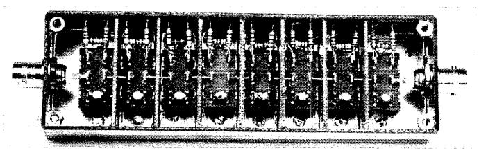
Fig. 4 — An inside view of the completed attenuator. Use of short, direct leads enhances the performance of the unit. Brass nuts soldered at each of the four corners allow machine screws to be used to secure the bottom cover. File one corner of each nut to permit a flat, two-sided fit within the enclosure.
