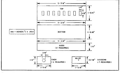
Fig. 2 -- Mechanical dimensions of the attenuator enclosure.
