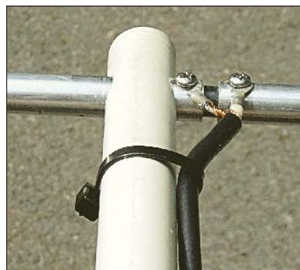
Figure 8 — A close-up of the junction of the support arm, the dipole element, and the connecting cable termination for portable operation. For a permanent installation, insert a stainless steel washer between the hook connector and the element and seal the junction.
