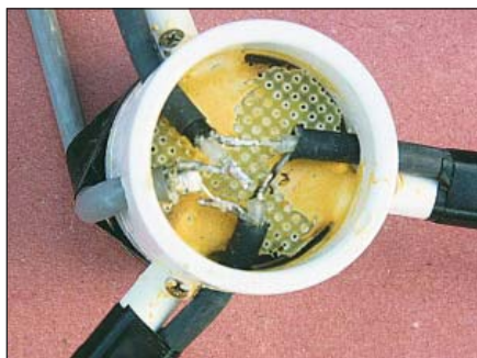
Figure 11 — The hub, support rods and the main junction of connecting cables and the \lambda/4 matching section before final sealing.
