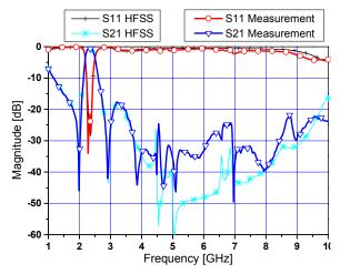
Fig. 5. Simulated and measured results of ring BPF with DGS and spur line.
