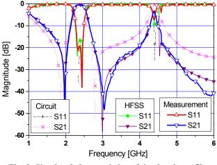
Fig. 3. Simulated characteristics of ring bandpass filter with DGS
