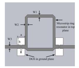
Fig. 1. Structure of the new ring bandpass filter
