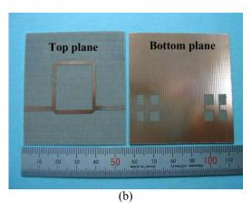
Fig. 6 Photos of the ring BPFs with (a) DGS (b) DGS and spur line
