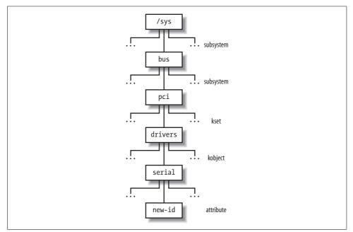
Figure 13-3. An example of device driver model hierarchy
