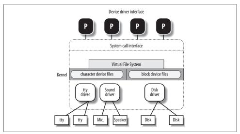
*Figure 1-4. Device driver interface*
