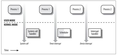
Figure 1-2. Transitions between User and Kernel Mode
