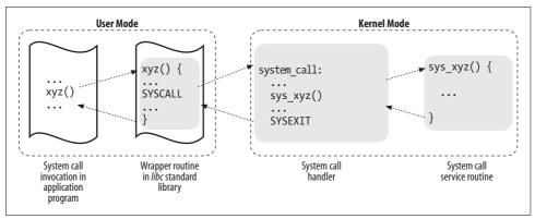
Figure 10-1. Invoking a system call
