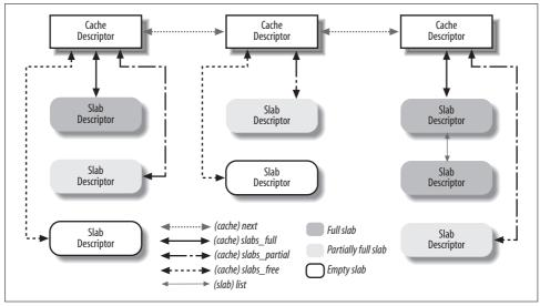
Figure 8-4. Relationship between cache and slab descriptors
