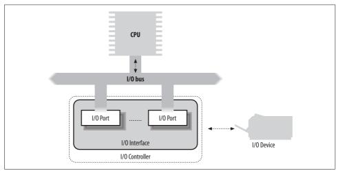
Figure 13-1. PC's I/O architecture
