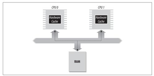
Figure 2-11. The caches in a dual processor
