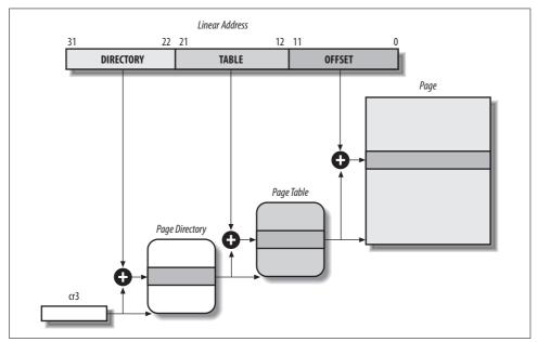
Figure 2-7. Paging by  $80 \times 86$  processors
