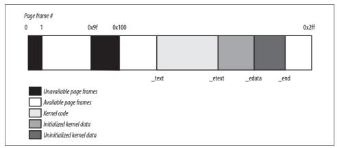
Figure 2-13. The first 768 page frames (3 MB) in Linux 2.6
