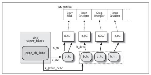
Figure 18-4. The ext2\_sb\_info data structure
