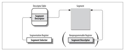
Figure 2-4. Segment Selector and Segment Descriptor
