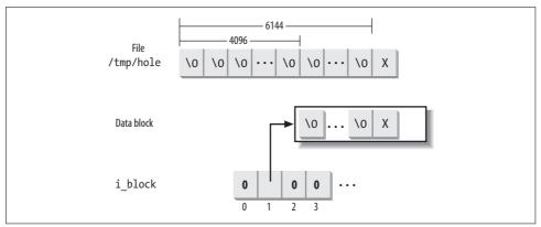
Figure 18-6. A file with an initial hole
