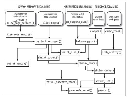
Figure 17-3. The main functions of the PFRA
