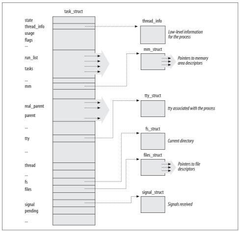
Figure 3-1. The Linux process descriptor
