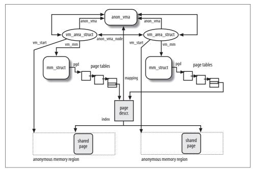
Figure 17-1. Object-based reverse mapping for anonymous pages
