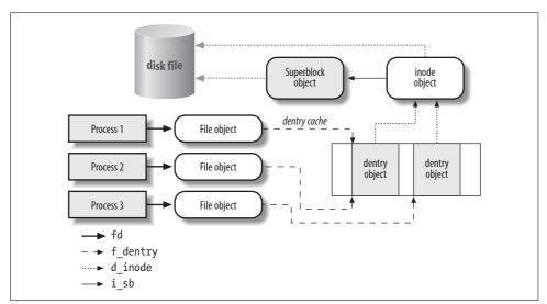
Figure 12-2. Interaction between processes and VFS objects
