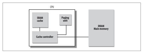
Figure 2-10. Processor hardware cache
