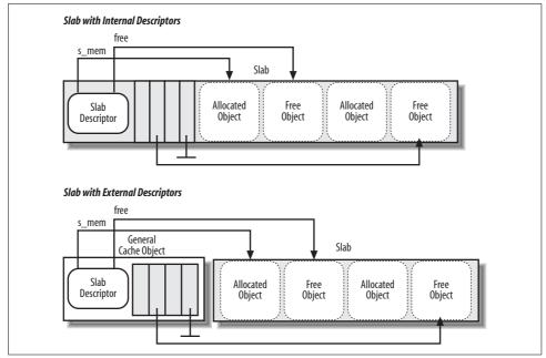
Figure 8-5. Relationships between slab and object descriptors
