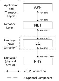
Figure 3. Communication system architecture for covert acoustical mesh networks
