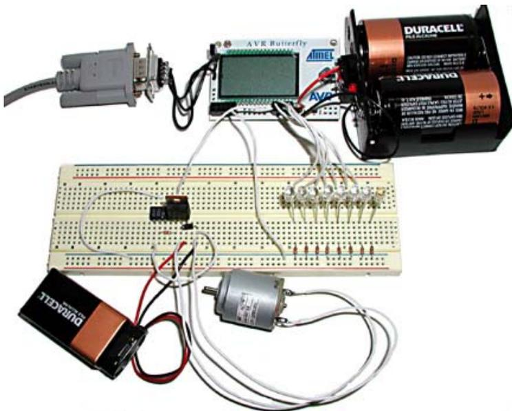
Figure 20: Motor Speed Control Hardware
