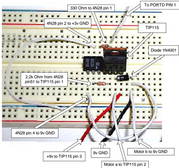
Figure 19: Motor Speed Control Breadboard Labeled
