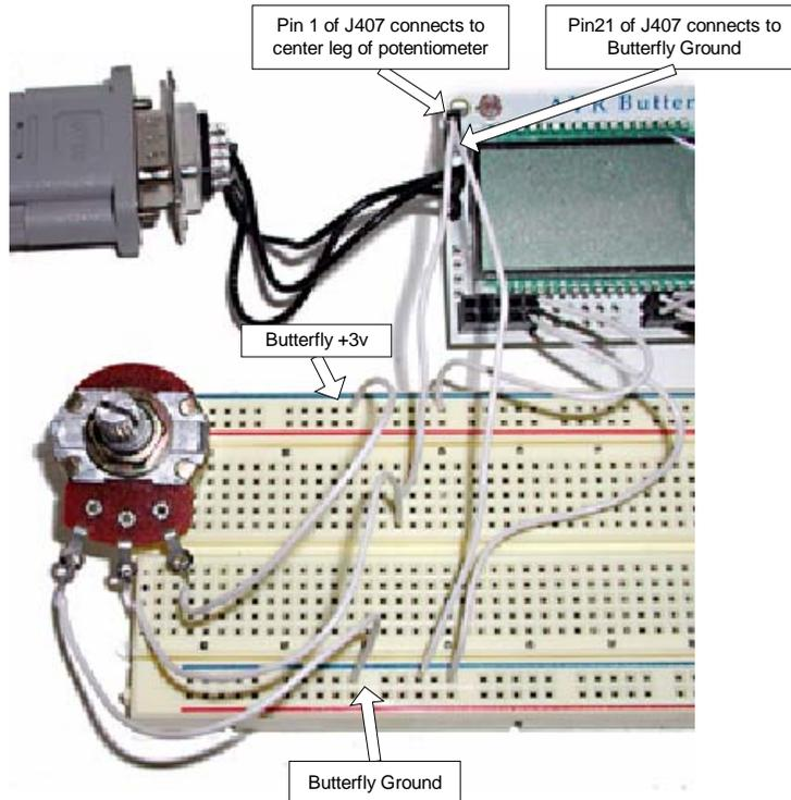
**Figure 29: Voltage measurement**
