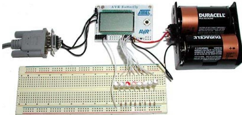
Figure 10: Hardware setup for Blinky.
