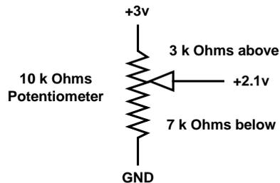
**Figure 28: Potentiometer Schematic**
