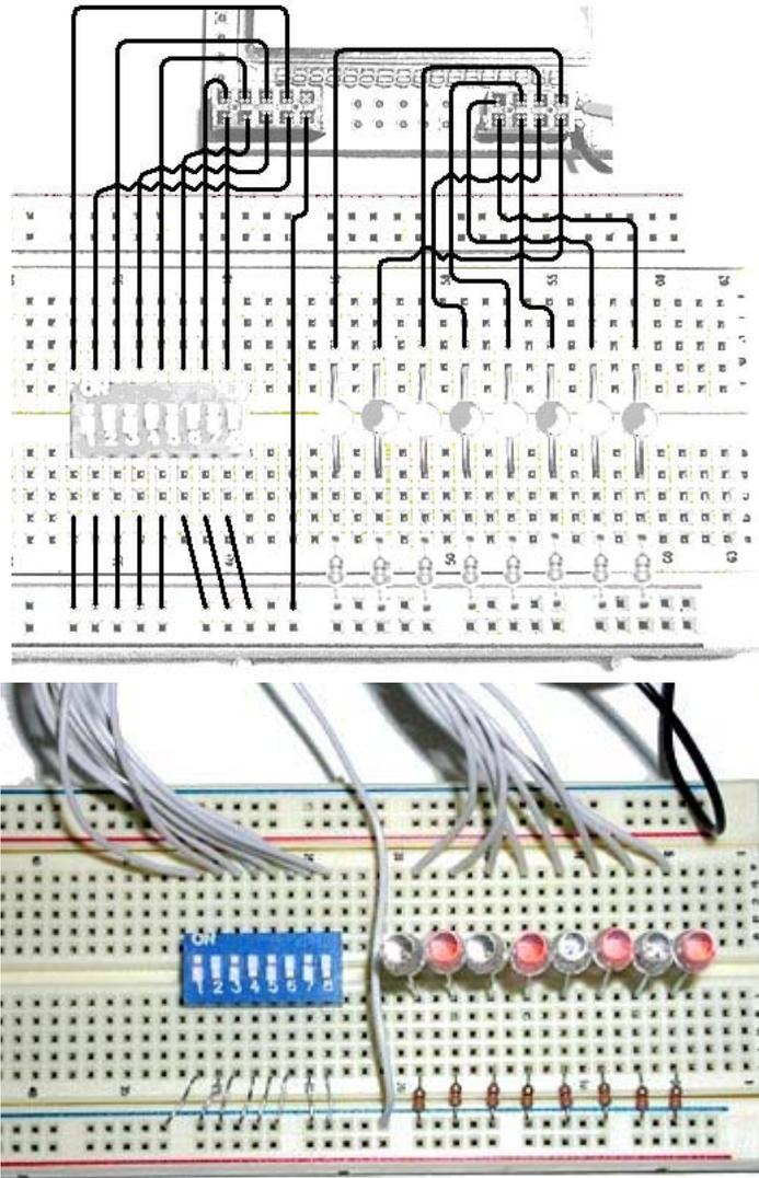
**Figure 14: Port I/O switch input and LED output**
