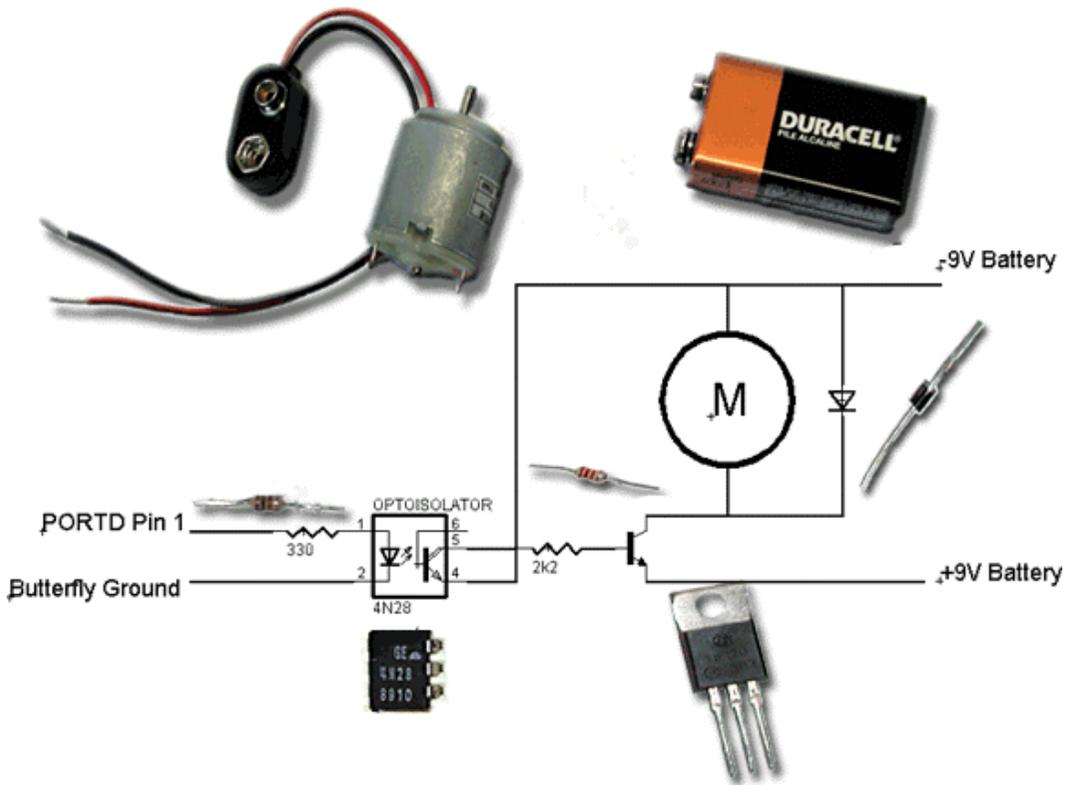
Figure 18: Motor Speed Control Schematic and Parts
