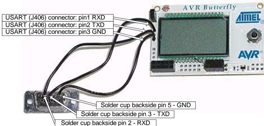
Figure 3: RS-232 connections.
