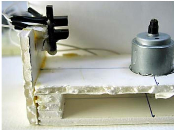
Figure 24: Opto Interrupter Glued on Motor Base
