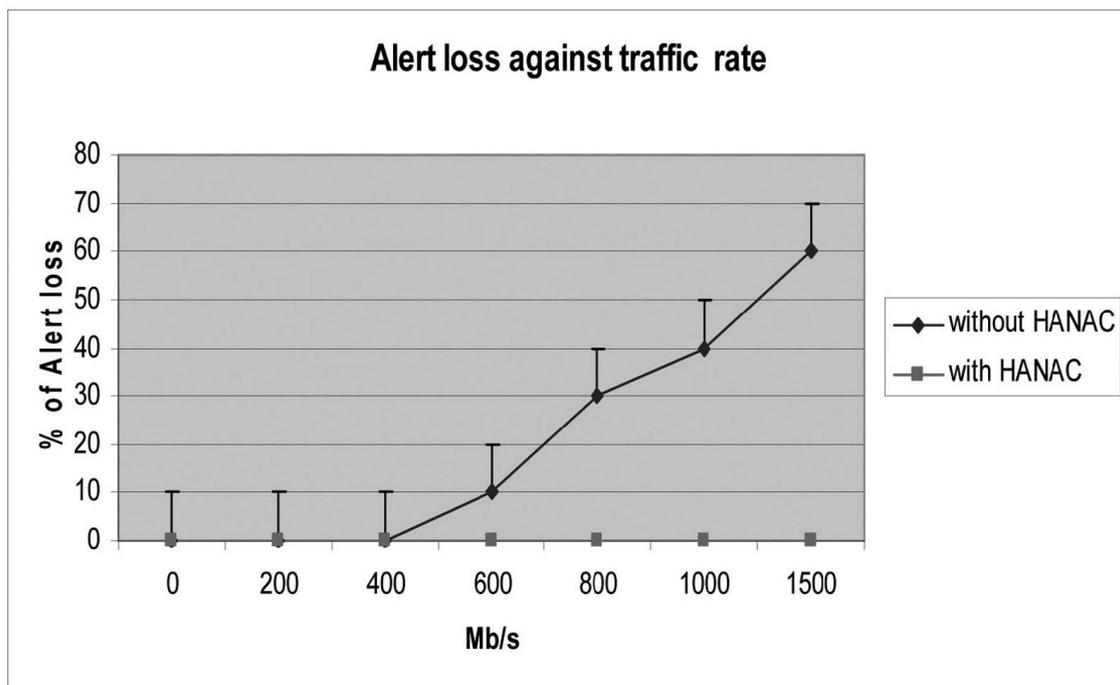
**FIGURE 11: LOSS AGAINST TRAFFIC RATE**
