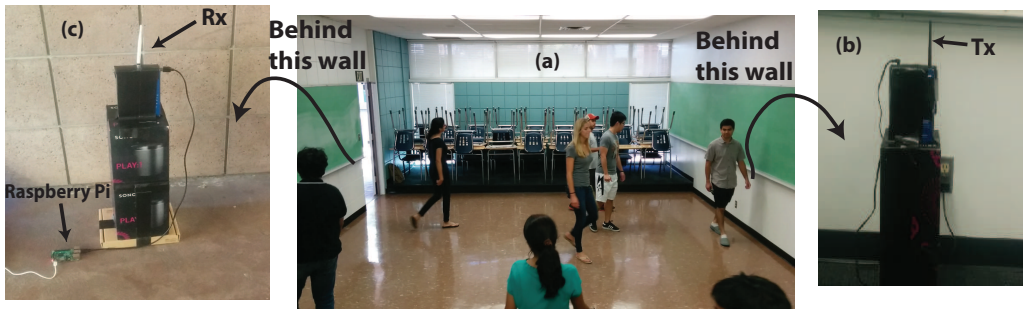
Fig. 6: (a) The first area of interest (Area 1), a closed classroom on our campus with wall made of concrete, where people are walking, (b) the Tx WiFi node located outside the classroom, behind one of the walls of the classroom as marked, and (c) the Rx WiFi node, along with the Raspberry Pi board that is used to control the data collection, which is located outside of the classroom behind the wall that is indicated.
