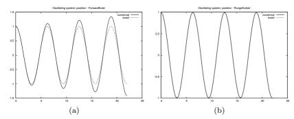
**Fig. E.4** Solution of an oscillating system (u'' + u = 0) formulated as system of two ODEs) by (a) the Forward Euler method with  $\Delta t = 2\pi/200$ ; and (b) the 4-th order Runge-Kutta method with  $\Delta t = 2\pi/20$ .
