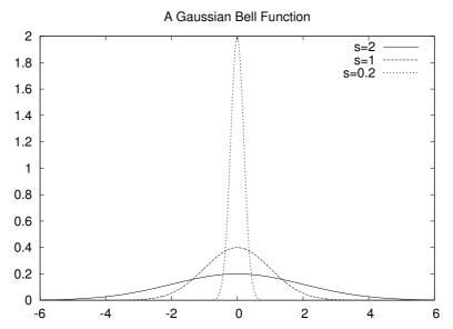
Fig. 5.7 Different shapes of a Gaussian function.
