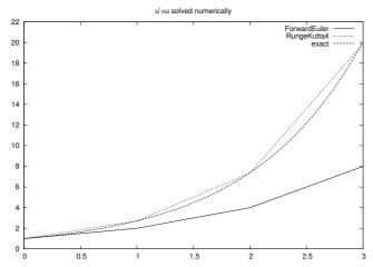
**Fig. E.2** Comparison of the Forward Euler and the 4-th order Runge-Kutta method for solving u' = u for  $t \in [0,3]$  and a long time step  $\Delta t = 1$ .
