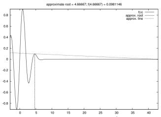
**Fig. A.2** Failure of Newton's method to solve  $e^{-0.1x^2}\sin(\frac{\pi}{2}x) = 0$ . The plot corresponds to the second root found (starting with x = 3).
