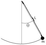
Fig. C.2 A pendulum with m = mass, L = length of massless rod and  $\theta = \theta(t) = \text{angle}$ .
