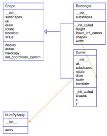
Fig. 9.8 UML diagram of parts of the shapes hierarchy. Classes Rectangle and Curve are subclasses of Shape. The darkest arrow with the biggest arrowhead indicates inheritance and is-a relationship: Rectangle and Curve are both also Shape. The lighter arrow indicates has-a relationship: Rectangle has a Curve, and a Curve has a NumP-yArray.
