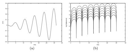
**Fig. D.5** Error plots for a test problem involving an oscillating system: (a) the error as a function of time; (b) the logarithm of the absolute value of the error as a function of time, where  $\Delta t$  is reduced by one half from one curve to the next one below.
