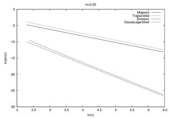
Fig. 9.4 The logarithm of the error versus the logarithm of integration points for integral  $5x^4$  computed by the Trapezoidal and Midpoint methods (upper two lines), and Simpson's rule and the Gauss-Legendre methods (lower two lines).
