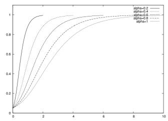
Fig. E.3 Solution of the logistic equation  $u' = \alpha u (1 - u/R)$  by the 4-th order Runge-Kutta method for various choices of  $\alpha$ .
