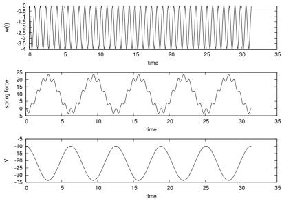
**Fig. D.4** Plot of the plate position w(t), the spring force (proportional to S(t)), and the position Y(t) for a test problem where  $w(t) = 2(\cos(8t) - 1)$ ,  $\beta = g = 0$ , m = k = 1,  $S_0 = 0$ ,  $\Delta t = 0.5236$ , and N = 600.
