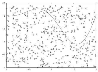
**Fig. 8.5** The "dart" method for computing integrals. When M out of N random points in the rectangle  $[0,2] \times [0,2.4]$  lie under the curve, the area under the curve is estimated as the M/N fraction of the area of the rectangle, i.e.,  $(M/N)2 \cdot 2.4$ .
