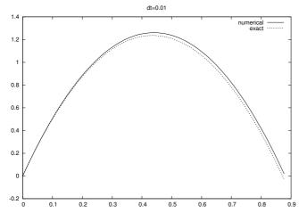
Fig. E.5 The trajectory of a ball solved as a system of four ODEs by the Forward Euler method.
