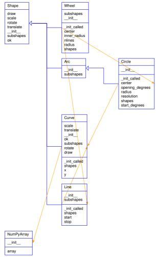
Fig. 9.9 This is a variant of Figure 9.8 where we display how class Wheel relates to other classes in the shapes hierarchy. Wheel is a Shape, like Arc, Line, and Curve, but Wheel contains Circle and Line objects, while the Circle and Line objects have a Curve, which has a NumPyArray. We also see that Circle is a subclass of Arc.
