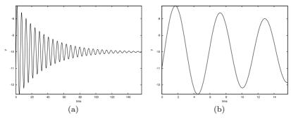
**Fig. D.3** Plot of the position of an oscillating box where the end point of the spring (w(t)) is given a sudden movement at t=0. Other parameters are m=k=1,  $\beta=0.1$ , g=0,  $S_0=0$ . (a) 1000 time steps; (b) 100 steps for magnifying the first oscillation cycles.
