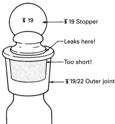
**FIGURE 4.2** A 19 nonstandard in a 19/22 standard taper joint.
