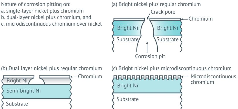
**Microdiscontinuous chromium** is the term applied to both microcracked and microporous chromium processes. **Microcracked chromium** can be achieved by modifying the formulation and/or the operating parameters of the chromium plating solution or, by using a highly-stressed nickel plating under the chromium, which induces microcracking in that chromium coating.
