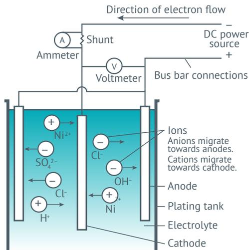
During electroplating, the positively charged metal ions discharge at the cathode (the component to be plated) depositing metal on the surface. The component being plated therefore receives a coating of metal. The reverse effect occurs at the anode and, with a soluble anode, metal ions are formed through dissolution.
