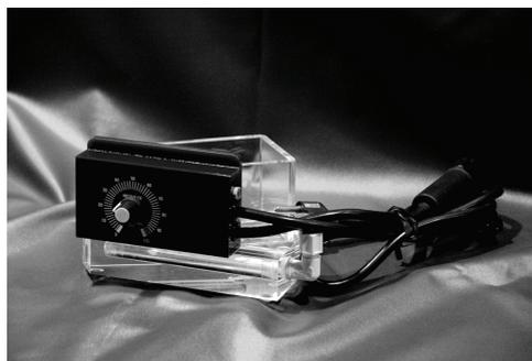
bright nickel baths. At the same time the panel can be examined for low current density darkness, brittleness or other defects. As the current density range on the Hull Cell panel is often broader than that on production components, the test may give early warning of potential problems, for example, the effects of impurities or a brightener imbalance. Measurements of throwing power are also possible using the Hull Cell.
