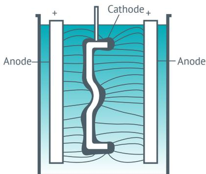
the solution. The complex relationship between these factors and metal distribution is termed the *throwing power*. Throwing power can be determined experimentally. Solutions exhibiting a positive value will be capable of reducing the variation in thickness between prominent and recessed areas. Conversely solutions with negative values, such as chromium plating solutions, may exhibit a greater thickness variation than would be expected based purely on geometric factors.
