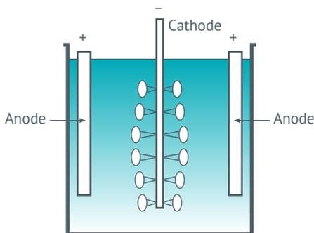
Good electrical contact with the anode bar must be maintained at all times. Anodes consisting of nickel metal are preferred in order to replenish the nickel ions and to simplify solution control. However, there are some occasions where insoluble anodes have to be employed. (see later section of this chapter)
