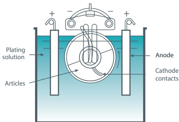
This type of immersed barrel is commonly transported through the various stages of the pre-treatment and plating cycle. Alternatively the barrel may be operated for the plating stage alone with the pre and post operations carried out in baskets.
